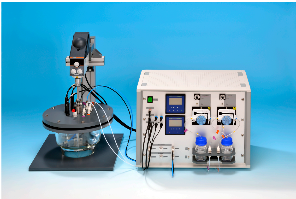
Figure 3.1: Advanced automated biogeochemical microcosm (MC) system used in experimental set up. A 4L borosilicate glass vessel with an air-tight seal and stir paddle has Eh, pH, and temperature sensors permanently installed from the lid to take measurements every 10 minutes. Measurements are taken and Eh, pH, and T can all be regulated automatically with the corresponding control unit.
