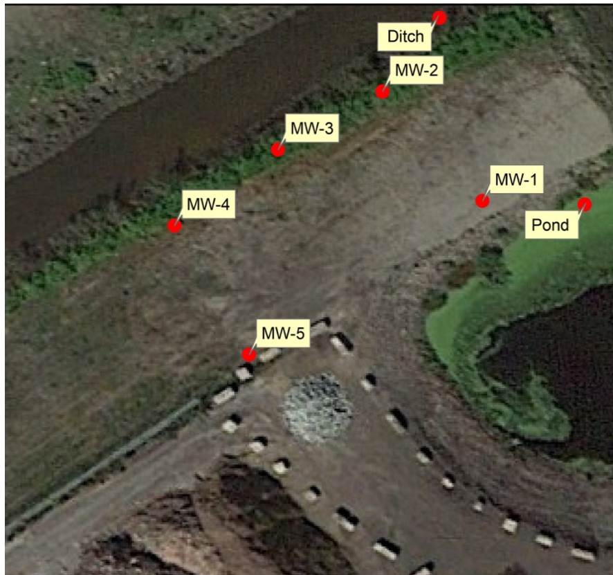
Figure 4.4: Location of groundwater wells installed by a consultant and used with their permission. Pressure transducers were installed in each of the indicated wells, as well as the ditch and collecting pond.
