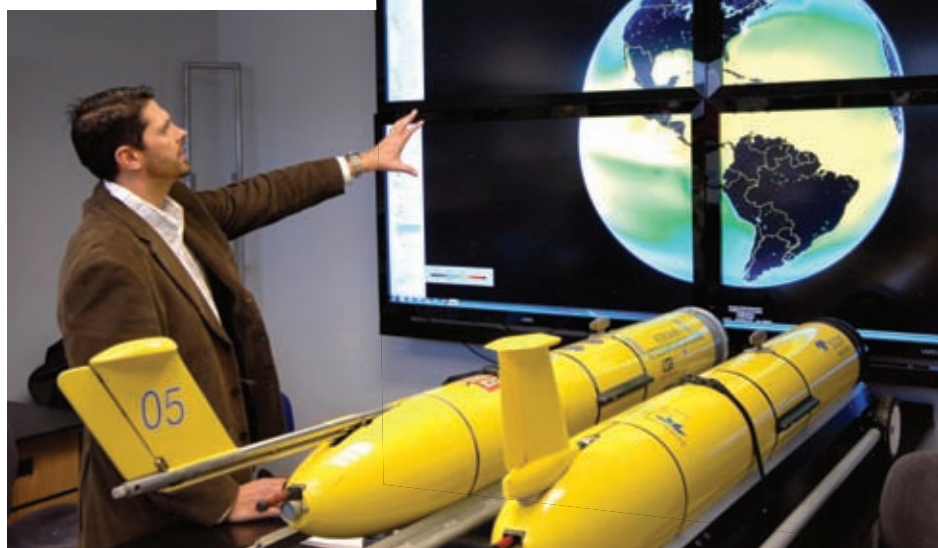
Oceanographer Matt Oliver is shown in the Global Visualization Lab at UD's Lewes campus with an autonomous underwater vehicle called a Slocum Electric Glider. The glider is a remotely operated robot that swims a sawtooth pattern and scans the ocean interior for traces of oil.
