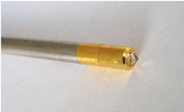
Fiber-optic MolecularEye ATR diamond probe from
