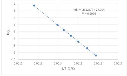
The graph shows a plot of the natural logarithm of k versus the inverse of the temperature (in kelvins), and the best-fit line through all of the points is quite linear. According to the Arrhenius theory, the slope is related to the activation energy:
