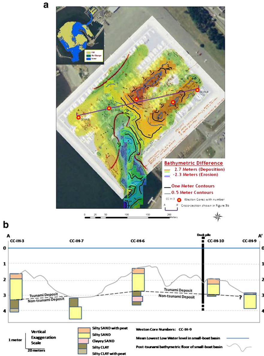
**Fig. 3.** (a) Areas of scour and fill in the Crescent City Harbor Small-Boat Basin determined by differencing multi-beam bathymetry collected by NOAA on March 16–21, 2011 and November 2008, superimposed on similar, more extensive raster image provided by Harbormaster (Stover Engineering, 2011); (b) cross section showing the post-tsunami bathymetry, sediment composition, and correlations between tsunami and non-tsunami deposits within the Small-Boat Basin.
