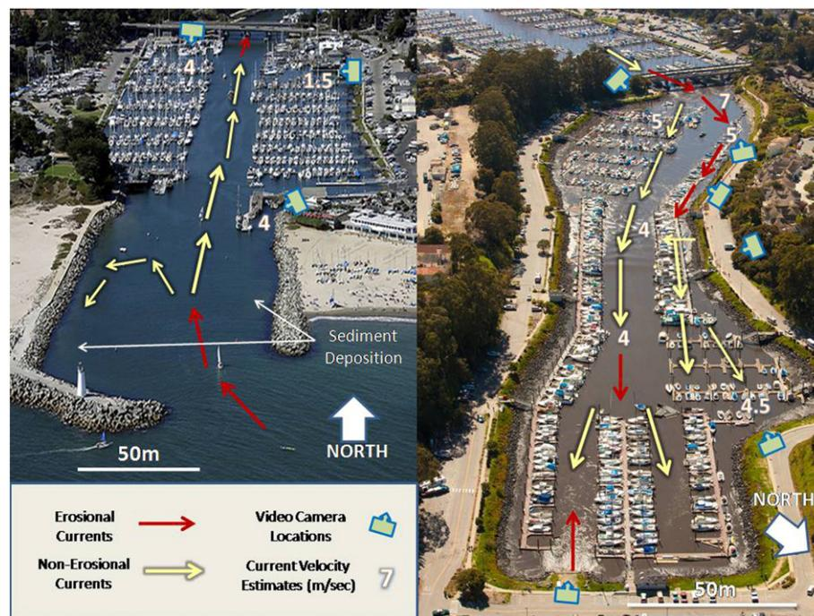
**Fig. 9.** Tsunami flow-regime map for Santa Cruz Harbor. Current directions and velocities, and areas of sediment erosion and deposition are based on observations of the various (30) ground-level and aerial video, pre- and post-tsunami bathymetry, and sediment analyses.
