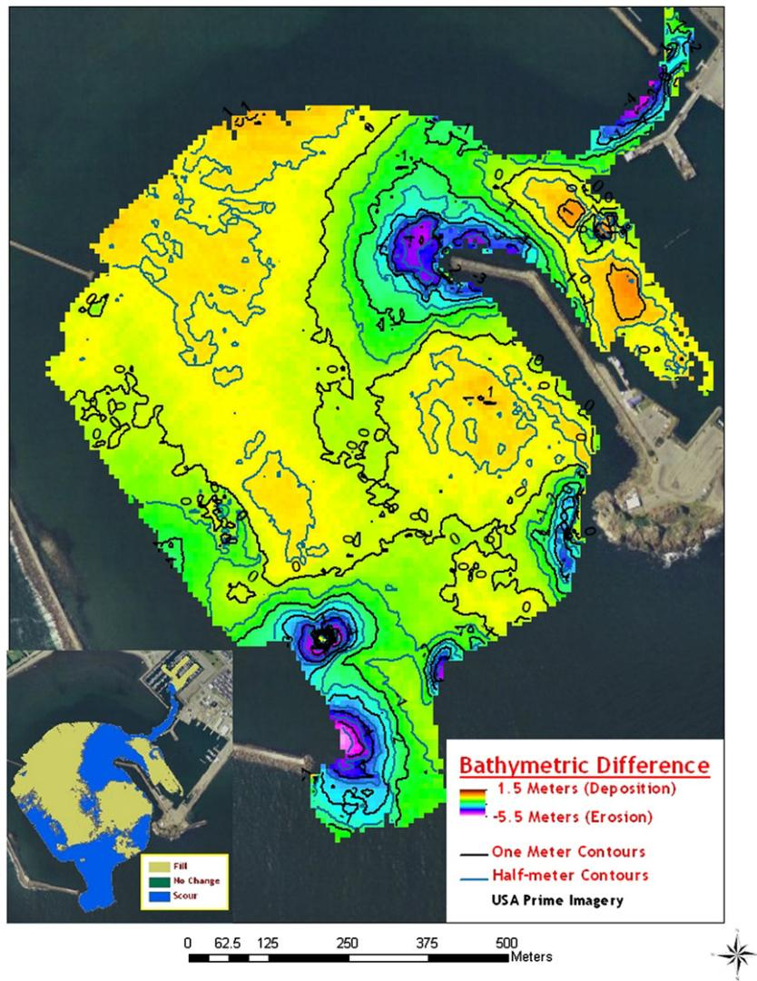
Fig. 4. Areas of scour and fill in the outer and middle portion of the Crescent City Harbor determined by differencing multi-beam bathymetry collected by NOAA on March 16–21, 2011 and November 2008.
