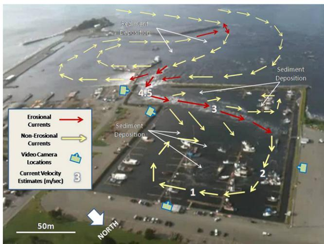
**Fig. 5.** Tsunami flow-regime map for Crescent City Harbor. Current directions and velocities, and areas of sediment erosion and deposition are based on observations of the various (30) ground-level and aerial video, pre- and post-tsunami bathymetry, and sediment analyses.
