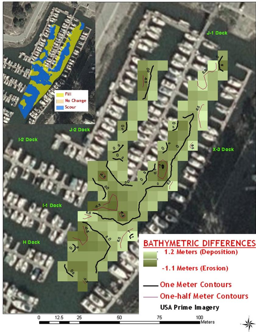
**Fig. 8.** Areas of scour and fill near the north end of the Santa Cruz Harbor determined by differencing Harbormaster soundings, collected on January 27–28, 2011, and February 21, 2011, with multi-beam bathymetry collected by NOAA on March 21, 2011.
