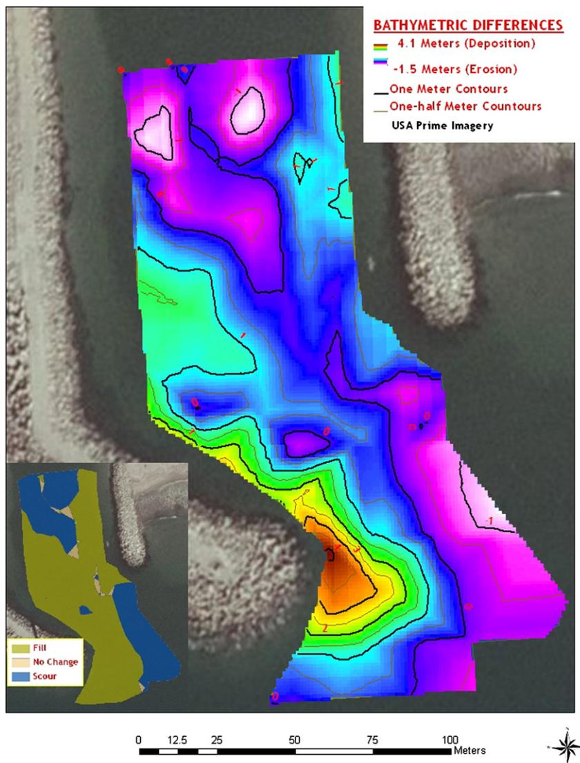
Fig. 7. Areas of scour and fill at Santa Cruz Harbor entrance, determined by differencing Harbormaster soundings collected on March 21, 2011 and February 23, 2011.
