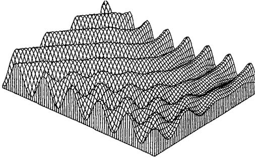
Figure 5. Instantaneous Water Surface Elevation Around Breakwaters.
