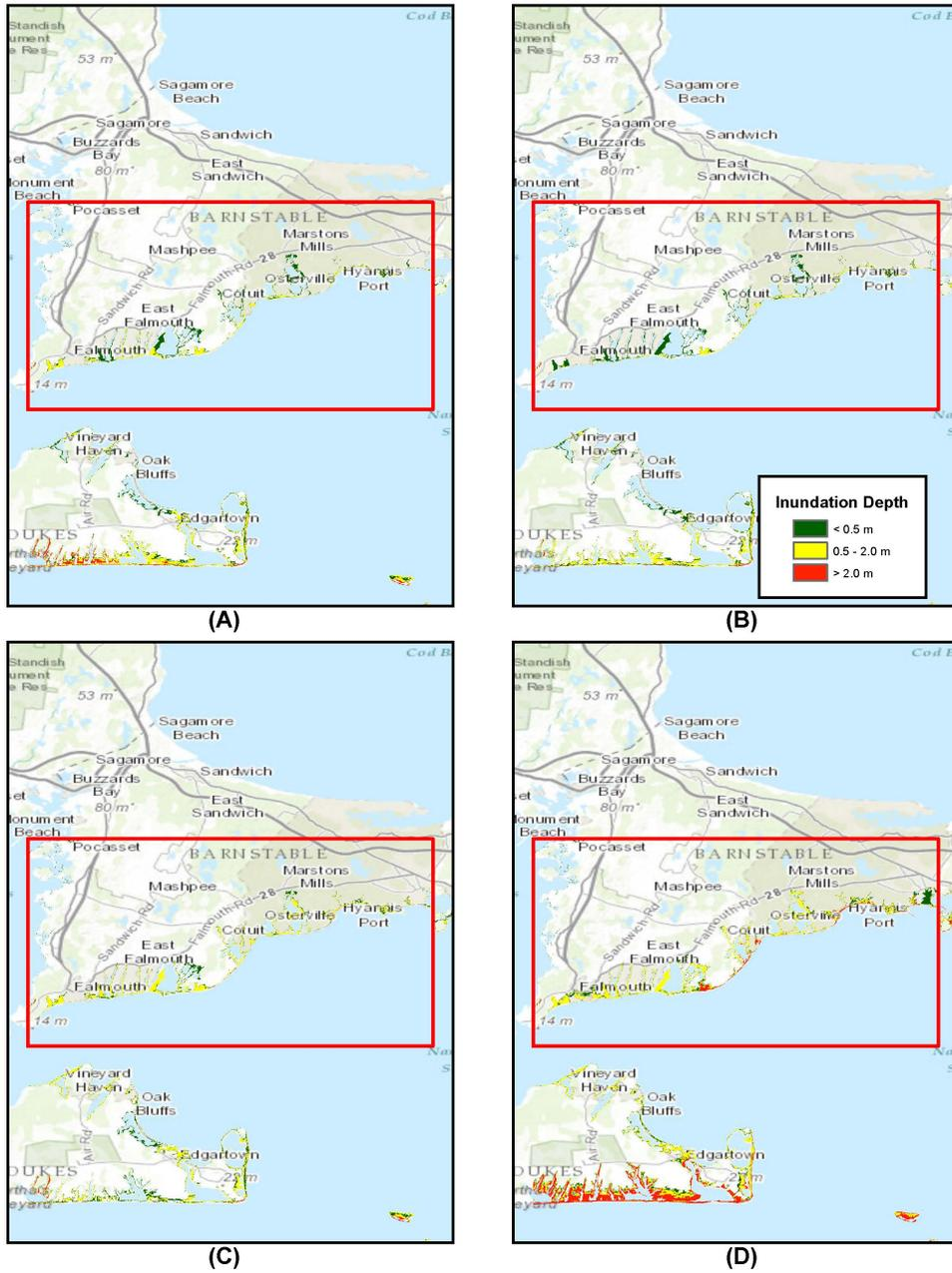
Figure 10: Inundation depth for NA\_1arc\_3 domain, A) SMF Envelope, B) Coseismic Envelope, C) CVV 80 km<sup>3</sup> slide, and D) CVV 450 km<sup>3</sup> slide. Red box depicts NA\_1arc\_3 domain boundaries.
