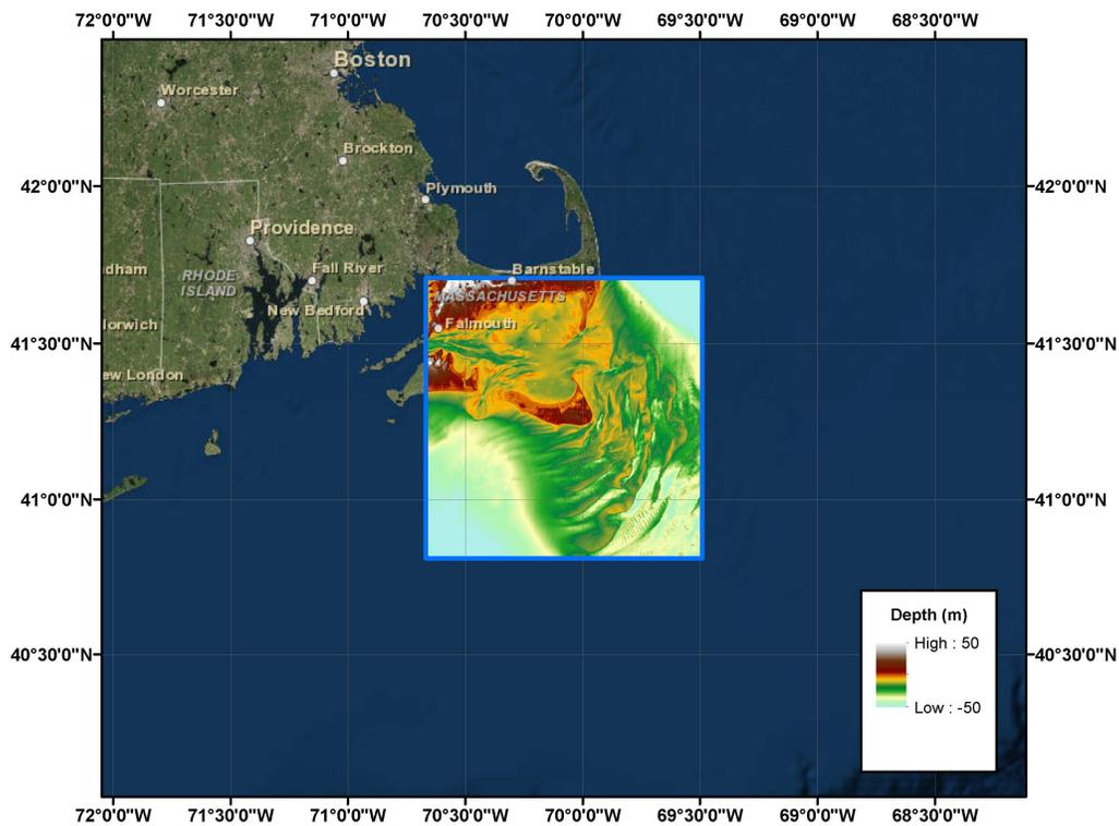
Figure 1: Location of the NGDC Nantucket DEM (Eakins et al, 2009). Color bar shows depth values in meters for areas inside of the DEM boundary.
