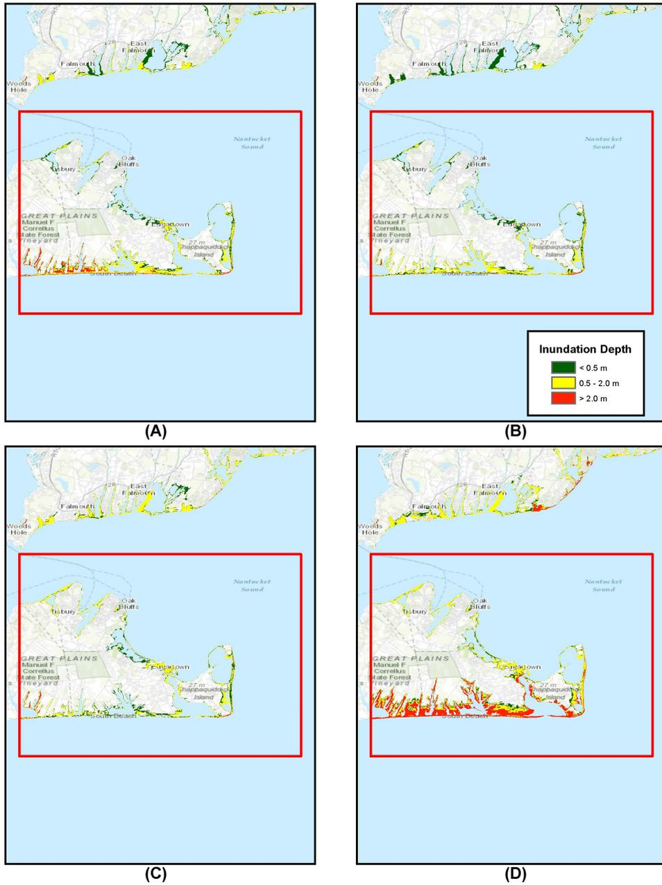
Figure 9: Inundation depth for NA\_1arc\_2 domain, A) SMF Envelope, B) Coseismic Envelope, C) CVV 80 km<sup>3</sup> slide, and D) CVV 450 km<sup>3</sup> slide. Red box depicts NA\_1arc\_2 domain boundaries.
