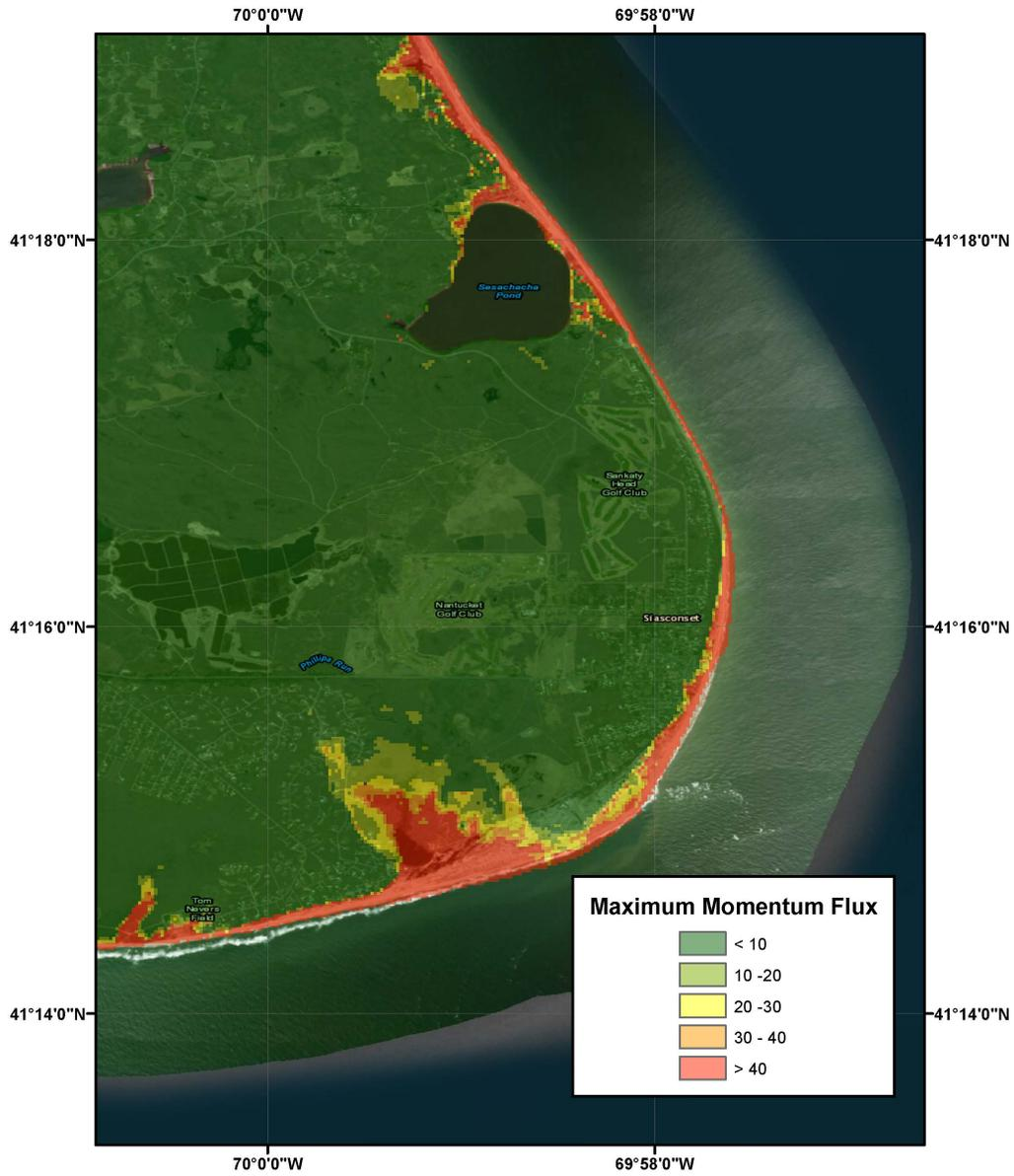
Figure 12: (Maximum Momentum Flux Map for the east of the Nantucket island during CVV ( $80 \text{ km}^3$  slide) tsunami (Colorbar values are in  $m^3/s^2$ ).
