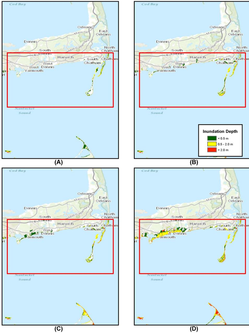
Figure 11: Inundation depth for NA\_1arc\_4 domain, A) SMF Envelope, B) Coseismic Envelope, C) CVV 80 km<sup>3</sup> slide, and D) CVV 450 km<sup>3</sup> slide. Red box depicts NA\_1arc\_4 domain boundaries.
