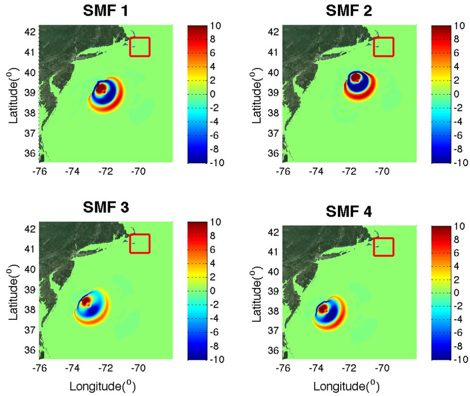
Figure 3: Location of Grid B and Nantucket DEM used in this project, and also the initial stage of SMF sources.
