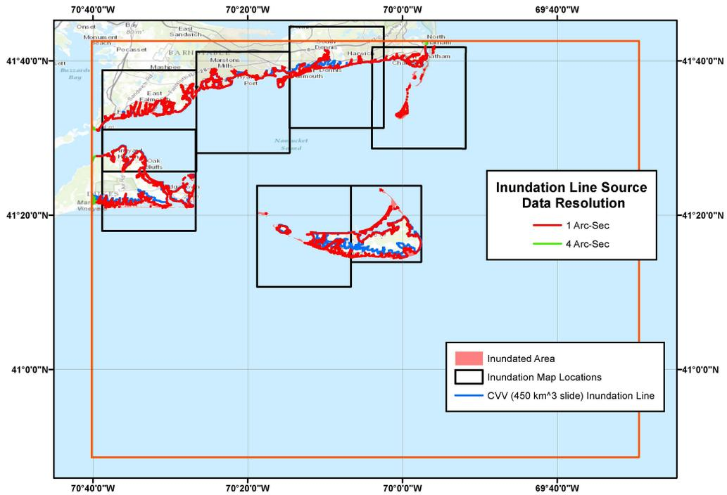
Figure 15: Tsunami inundation line for Nantucket NGDC DEM area based on tsunami sources simulated in this project. The blue boxes show the location of the inundation maps discussed in Section 5.
