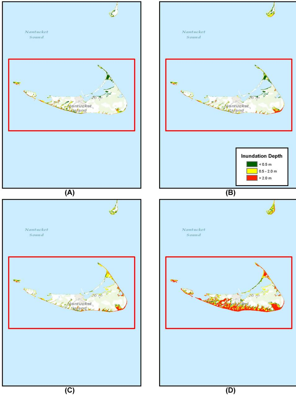
Figure 8: Inundation depth for NA\_1arc\_1 domain, A) SMF Envelope, B) Coseismic Envelope, C) CVV 80 km<sup>3</sup> slide, and D) CVV 450 km<sup>3</sup> slide. Red box depicts NA\_1arc\_1 domain boundaries.
