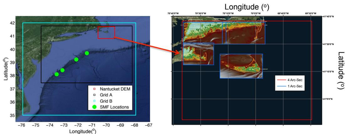
Figure 5: The sequence of grid nesting. The figure on the top left depicts the Grid A and B as well as the location of the Nantucket DEM. The figure on the right show the 1 arc-sec grids described in Table 1.
