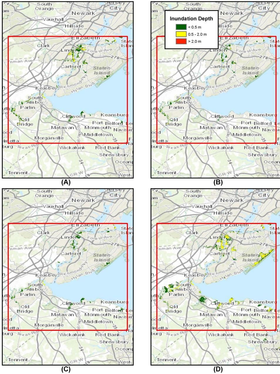
Figure 11: Inundation depth for NJ\_1arc\_4 domain, A) SMF Envelope, B) Coseismic Envelope, C) CVV 80 km<sup>3</sup> slide, and D) CVV 450 km<sup>3</sup> slide. Red box depicts NJ\_1arc\_4 domain boundaries.
