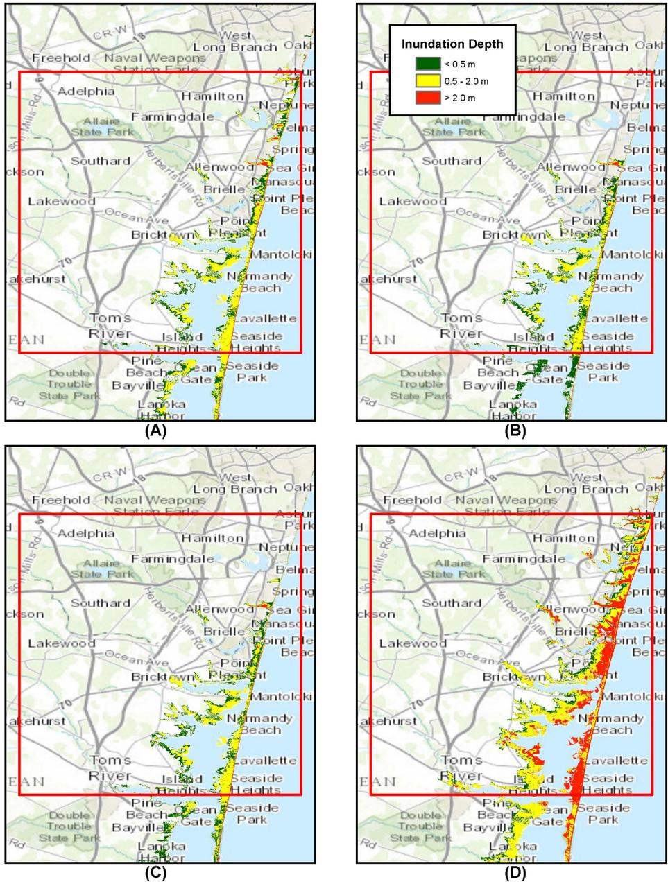
Figure 9: Inundation depth for NJ\_1arc.2 domain, A) SMF Envelope, B) Coseismic Envelope, C) CVV 80 km<sup>3</sup> slide, and D) CVV 450 km<sup>3</sup> slide. Red box depicts NJ\_1arc.2 domain boundaries.
