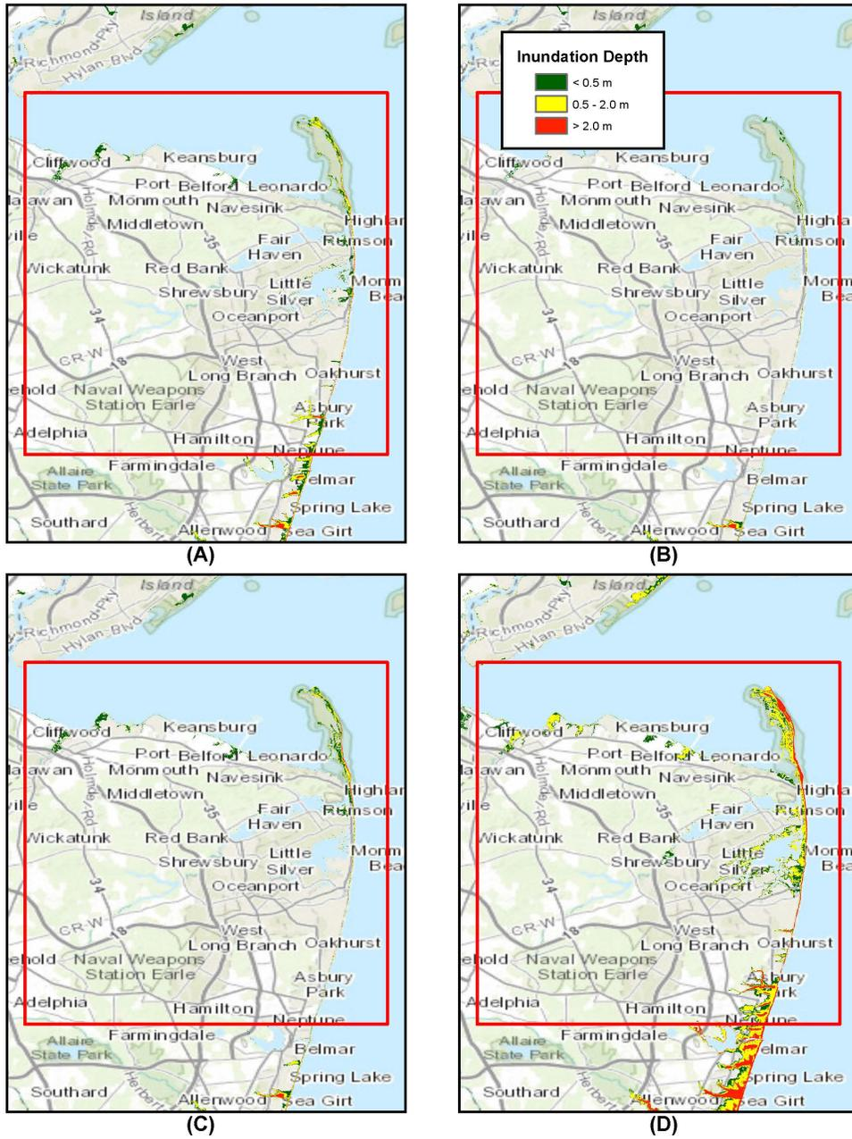
Figure 10: Inundation depth for NJ\_1arc\_3 domain, A) SMF Envelope, B) Coseismic Envelope, C) CVV 80 km<sup>3</sup> slide, and D) CVV 450 km<sup>3</sup> slide. Red box depicts NJ\_1arc\_3 domain boundaries.
