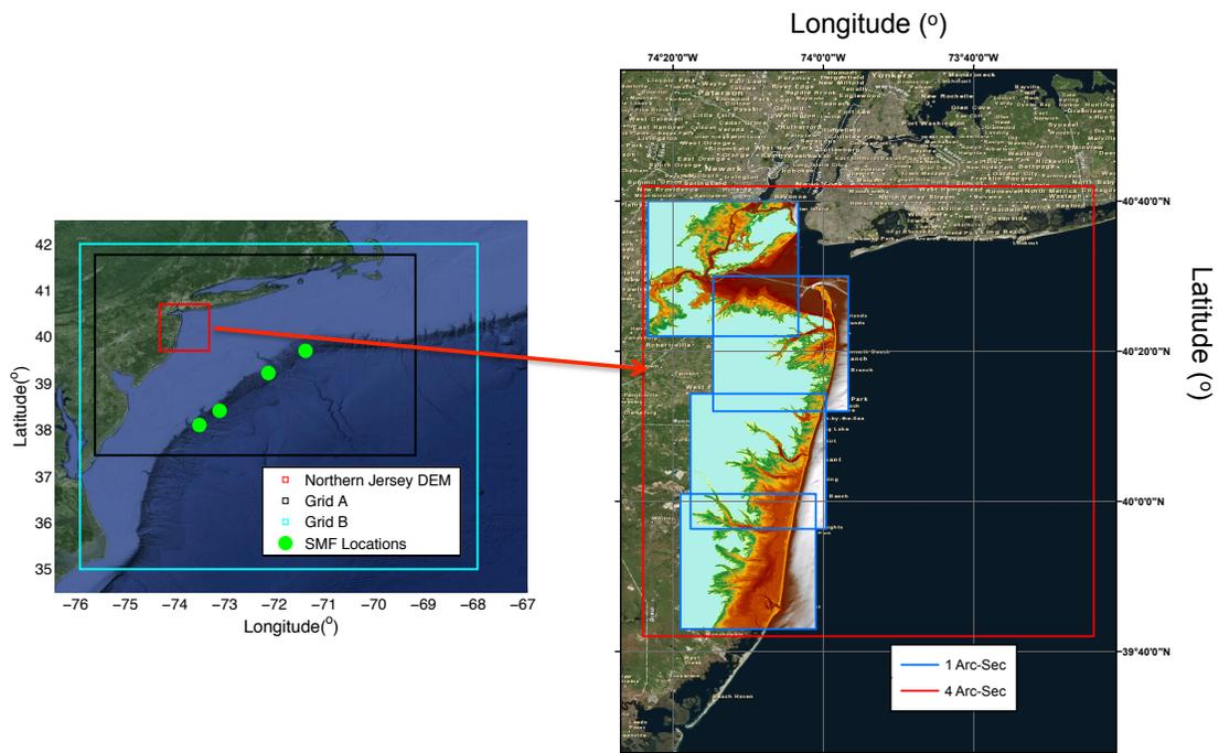
Figure 5: The sequence of grid nesting. The figure on the top left depicts the Grid A and B as well as the location of the Northern New Jersey DEM. The figure on the right show the 1 arc-sec grids described in Table 1.
