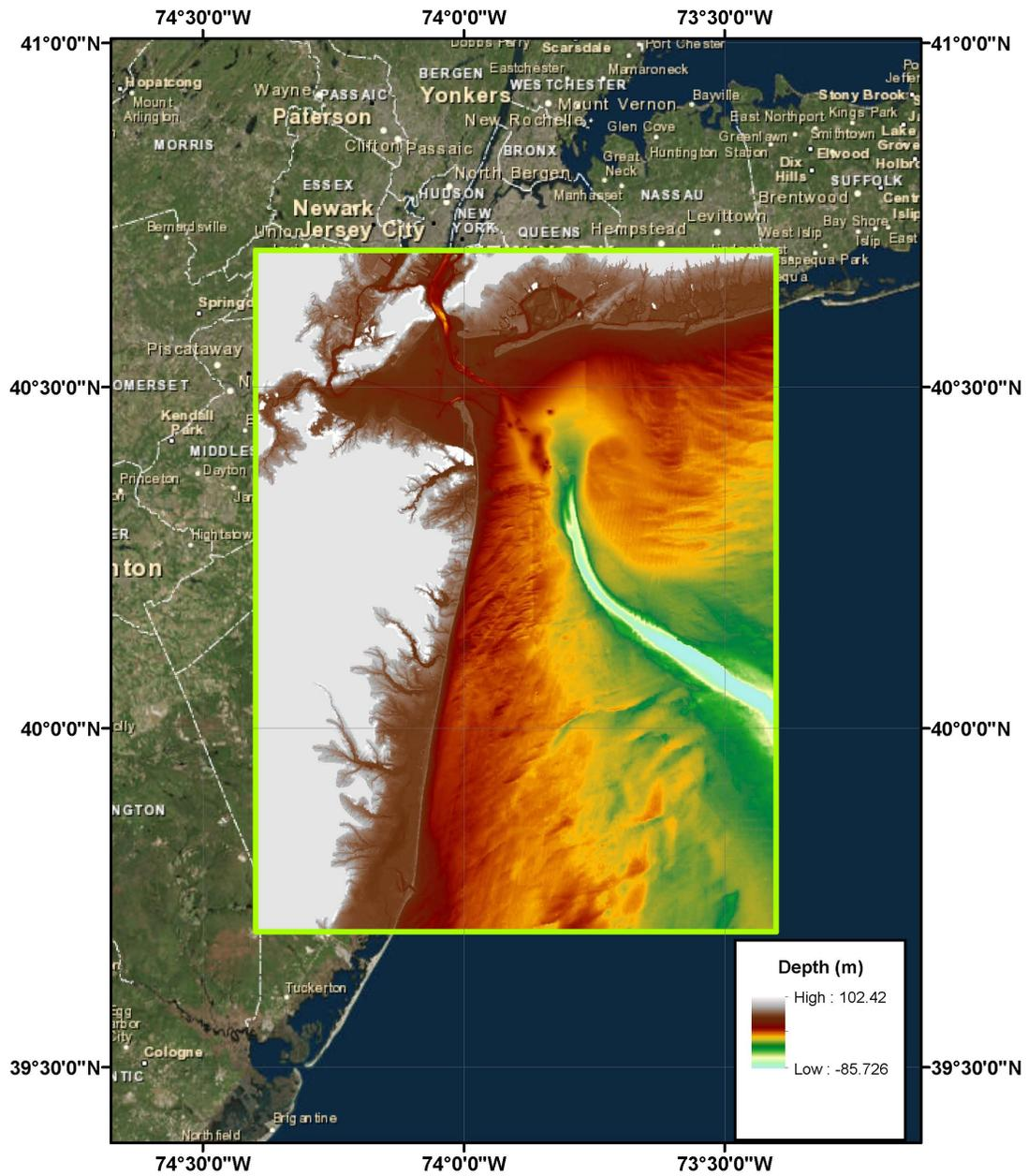
Figure 1: Location of the Northern New Jersey DEM. Color bar shows depth values in meters for areas inside of the DEM boundary.
