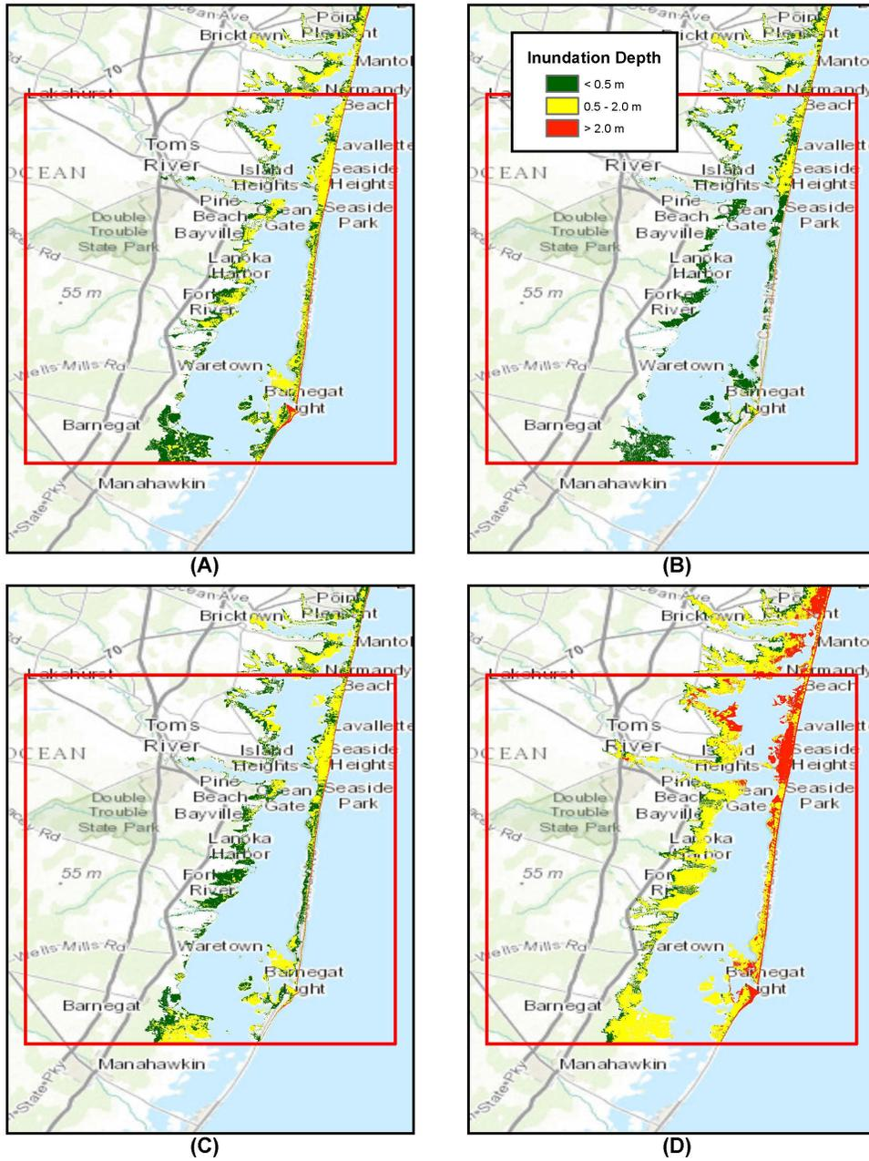
Figure 8: Inundation depth for NJ\_1arc\_1 domain, A) SMF Envelope, B) Coseismic Envelope, C) CVV 80 km<sup>3</sup> slide, and D) CVV 450 km<sup>3</sup> slide. Red box depicts NJ\_1arc\_1 domain boundaries.
