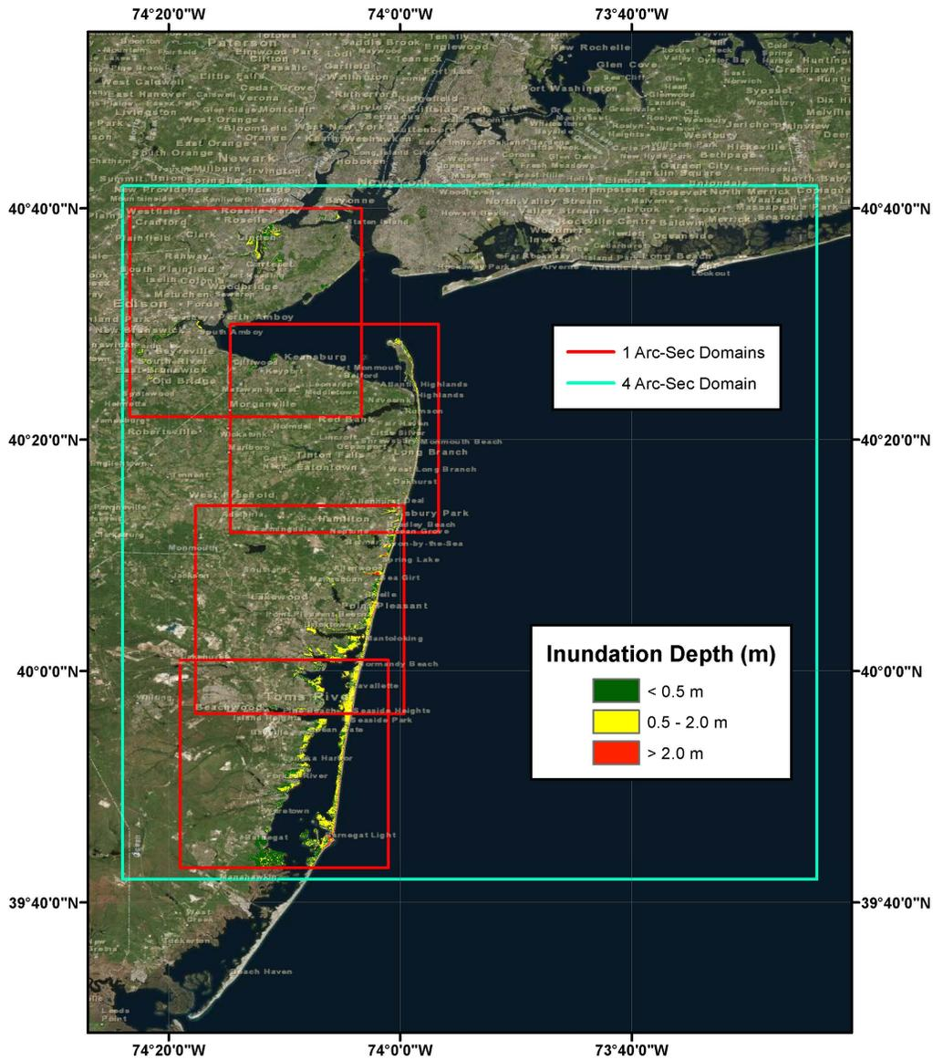
Figure 7: CVV 80 km<sup>3</sup> slide Inundation Map for the Northern New Jersey DEM with 4 arc-second resolution. Red squares depicts the 1 arc-second resolution domains
