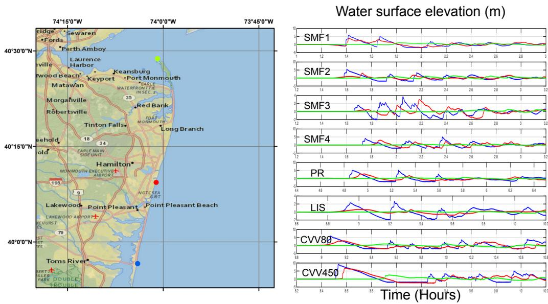
Figure 6: Recorded surface elevation for gauges located in different locations in Northern New Jersey DEM, Seaside Heights (Blue), Spring Lake (Red), and Sandy Hook, NJ (Green).
