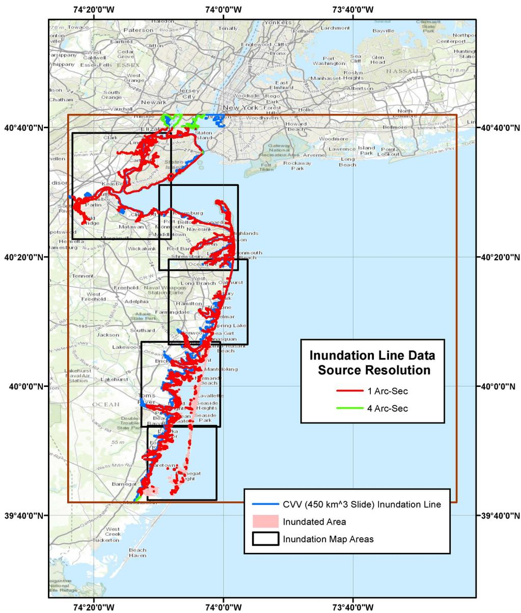
Figure 15: Tsunami inundation line for Northern New Jersey DEM area based on tsunami sources simulated in this project. The blue boxes show the location of the inundation maps discussed in Section 5.
