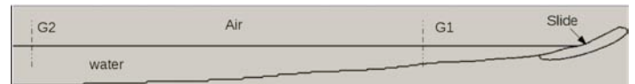
Fig. 2 : Initial conditions for Thetis 2D simulations. Numerical gages G1, G2, G3 (not represented here) located respectively 10 km, 45 km and 100 km off shore.
