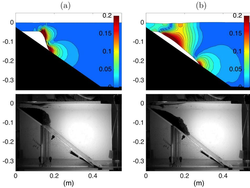
Figure 2. Comparison of model simulations of deforming slide tsunami generation and glass bead experiments (see Grilli et al., 2016c). This was selected as Benchmark #4 of workshop (<http://www1.udel.edu/kirby/landslide/index.html>).
