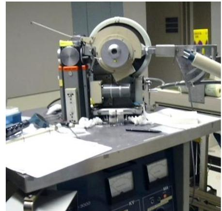
For XRDs with a full cabinet enclosure, operators are advised to conduct x-ray leakage surveys on a periodic basis. There is no requirement to record the result of their survey. Enclosure cabinets have been found to be effective and reliable at confining x-rays.
