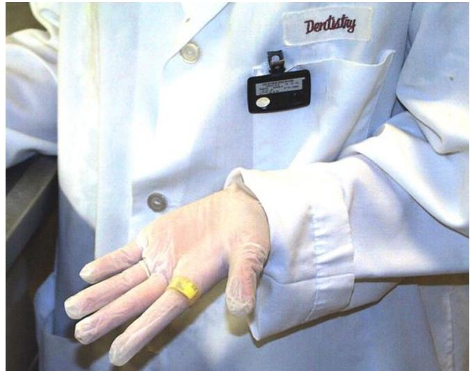
The dosimeters do not protect a worker from radiation exposure. They will not provide any visible or audible warning when being exposed to radiation. They are essential, however, in tracking a worker's radiation dose and confirming that occupational dose limits are not exceeded.
