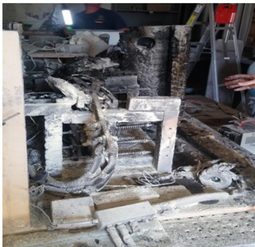
Fire damage at Spencer Lab from a lithium-ion battery test stand
