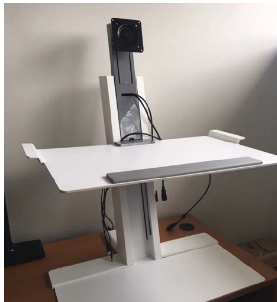
Sample Quickstand unit in the standing position.
