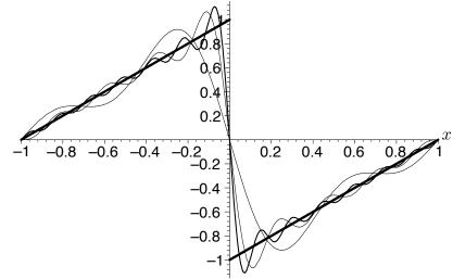
In increasing order of thickness: Fourier series keeping the first three, eight, and, thirteen terms in the series, as well as f(x) vs. x for L = 1.
