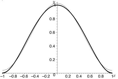
In increasing order of thickness: Fourier series keeping the first one, two, and, three terms in the series, as well as f(x) vs. x for L = 1.
