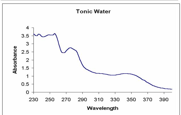
Figure 2-3. Absorbance spectrum of Schwepps tonic water, undiluted from the bottle.
