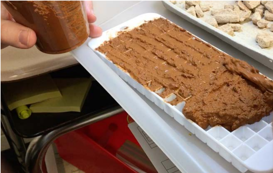
Fig. 3: Filling mini ice cube trays with mudbrick mixtures. Image credit: Merry Ostheimer
