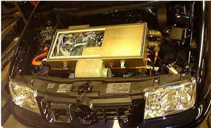
**Figure 3. Electric Drive System Installed**
