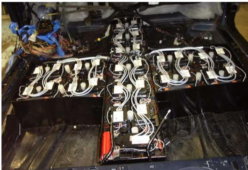
**Figure 4. Battery Installed**
