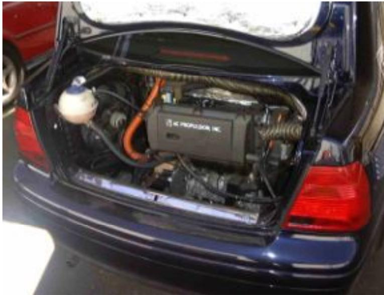
**Figure 7. APU Installed**
