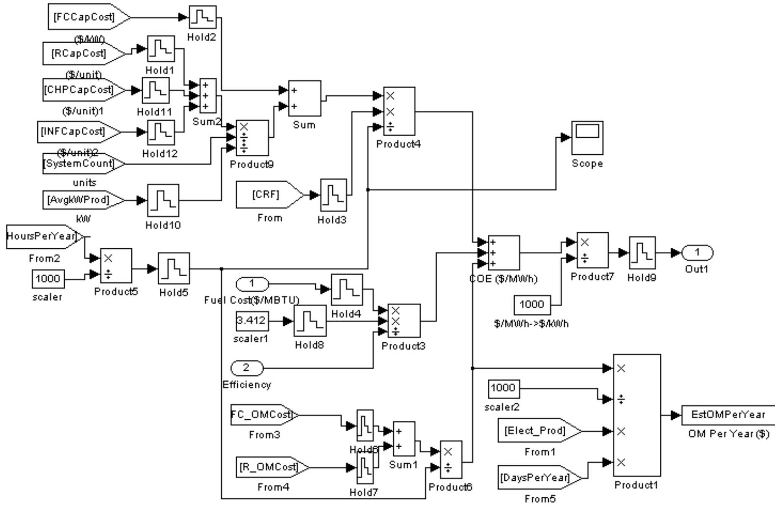
Figure 5: CETEEM Hot Water Cogeneration Submodel (Residential Example)
