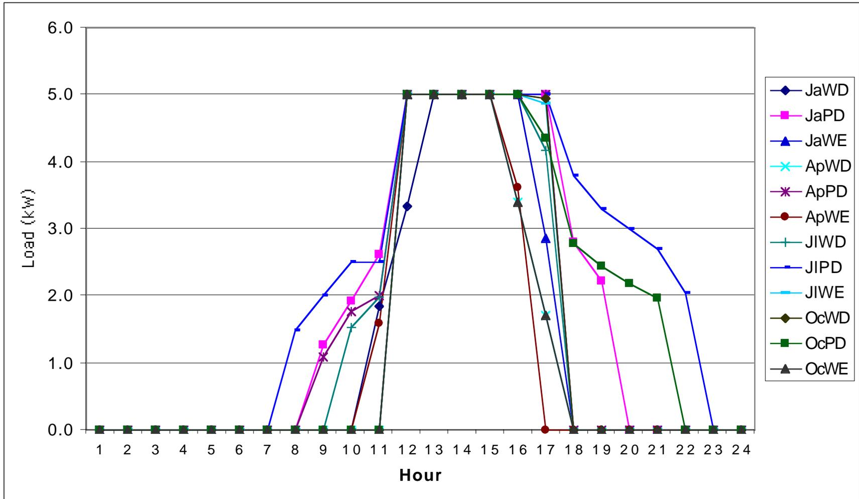
Figure 10: California Large Residential Site Modified Fuel Cell Load Patterns for FCV Net Metering
