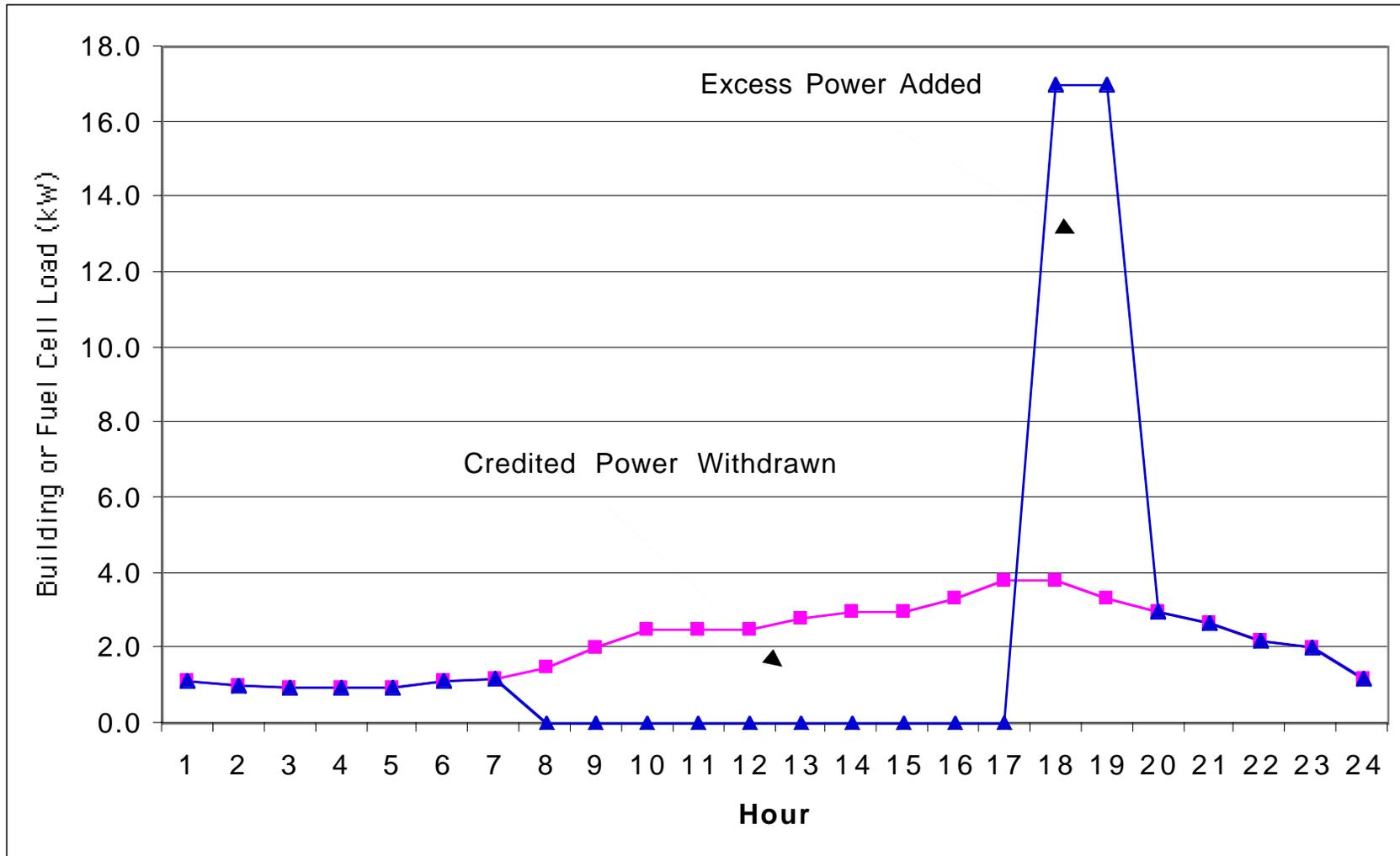
Figure 9: California Large Residential Site Modified Fuel Cell Load Patterns for 5 kW Stationary Fuel Cell Net Metering
