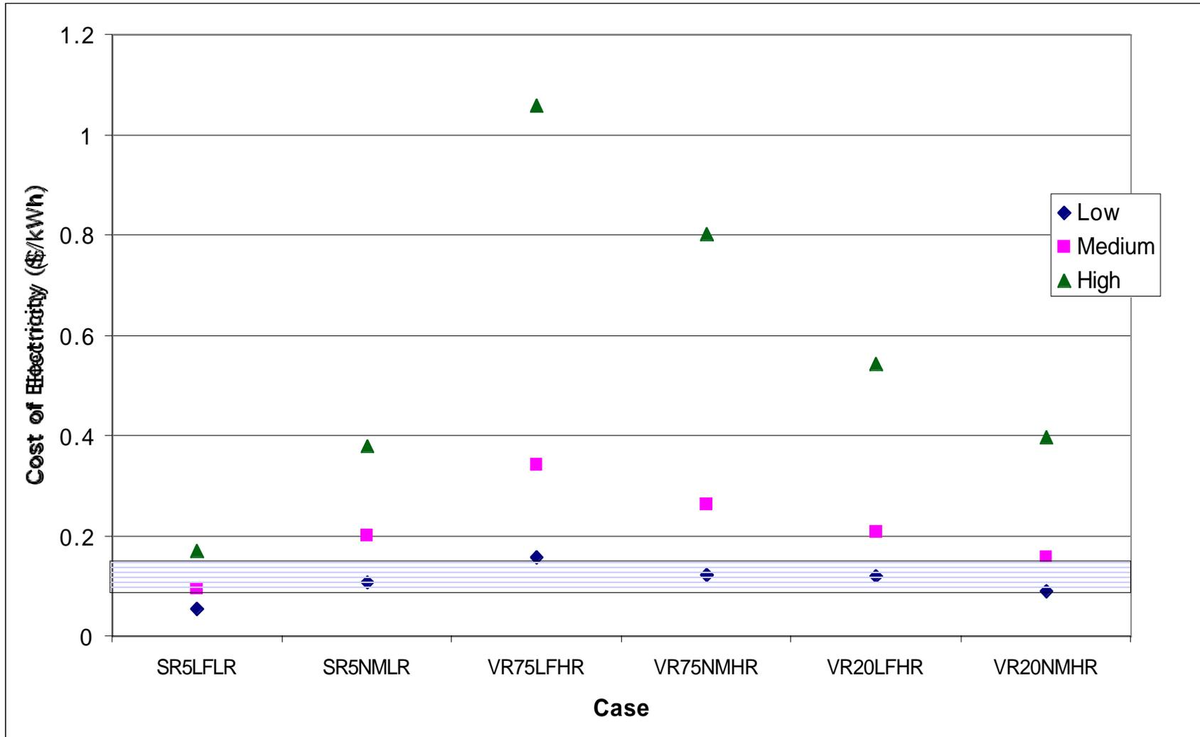
Figure 20: Cost of Electricity for Fuel Cell Operation in Office Building Setting Cases
