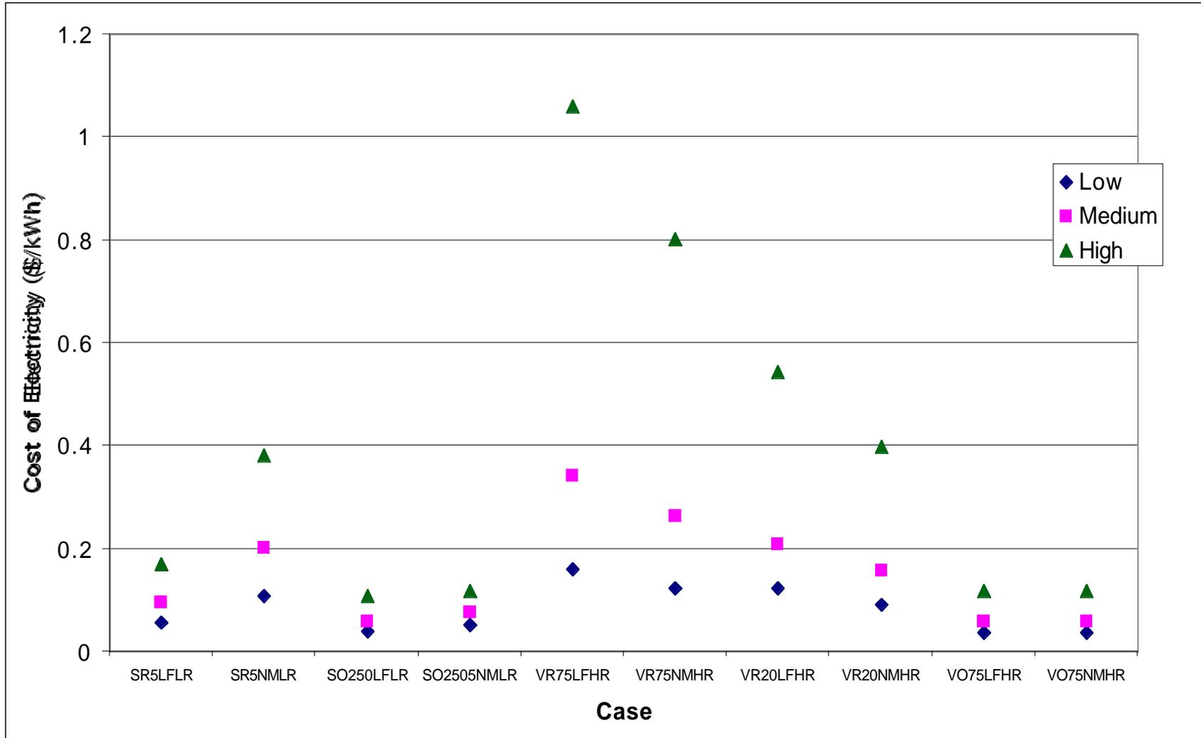
Figure 19: Cost of Electricity for Fuel Cell Operation in Residential Setting Cases
