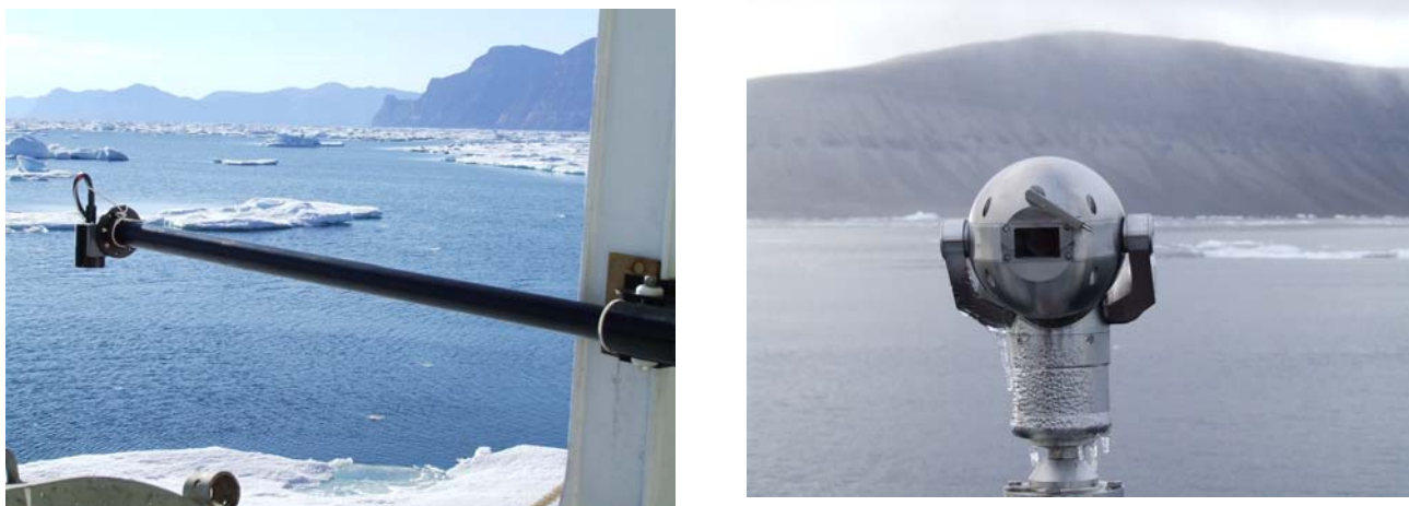
Figure 9. Cameras used to photograph the ice in the ship's path. That at the left is down-looking and provides images for measurement of ice thickness. That at the right photographs floes ahead of the ship before their impact.
