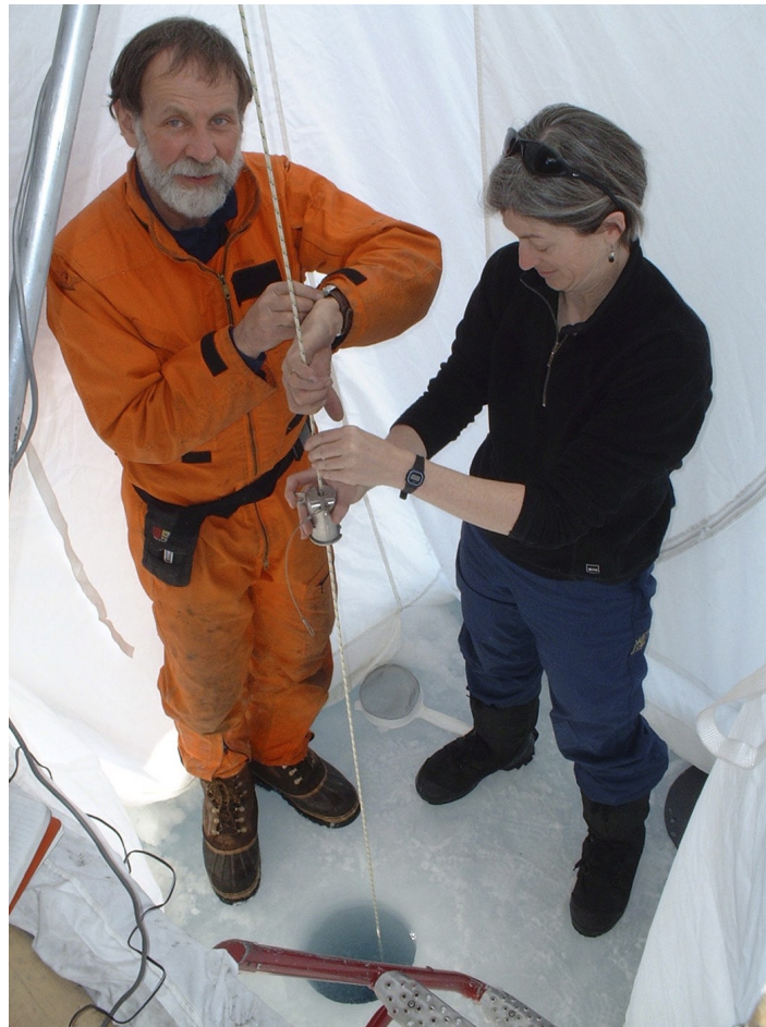
Launching the messenger to trip Niskin bottles in the central Arctic May 2002. Jamie Morison left, Kelly Falkner right. Photo by Jim Haffey.
