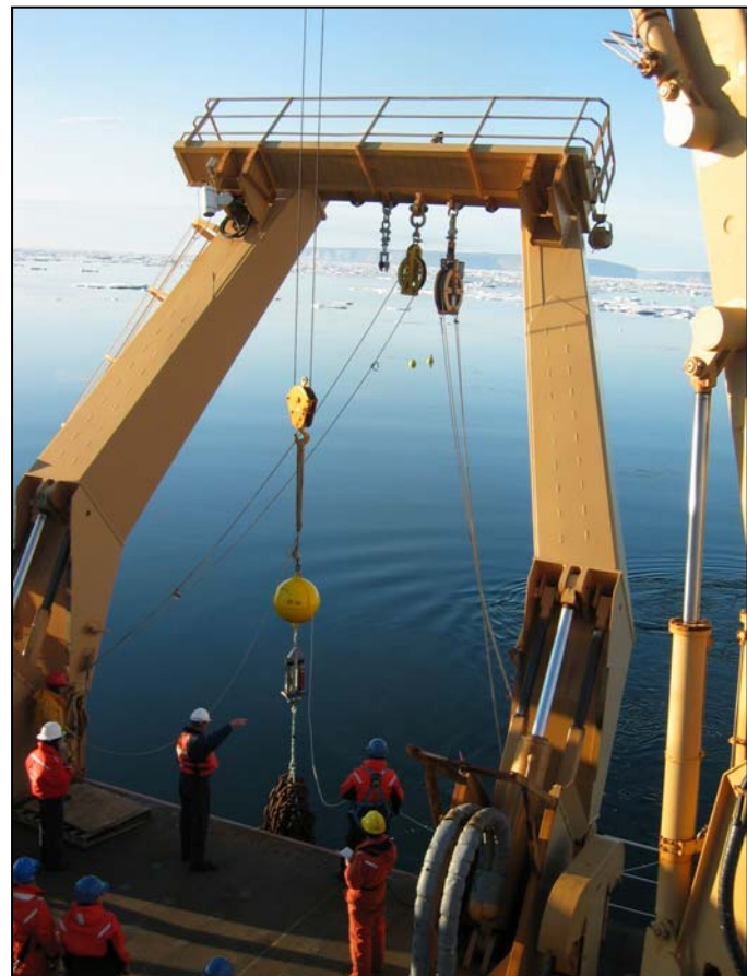
Figure 14. The final lift (float, tandem release assembly, drop line and anchor clump) of an ice-thickness mooring is shown on the crane, prior to its drop to the sea floor. Mooring floats appear in the background.
