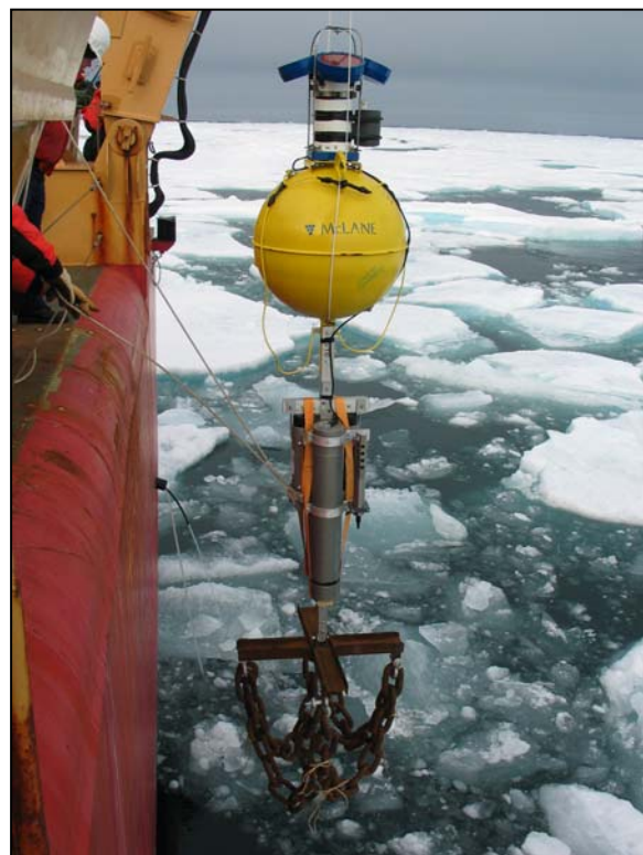
Figure 12. A long-range ADCP ready for deployment via the A-frame of USCGC Healy in August 2003.
