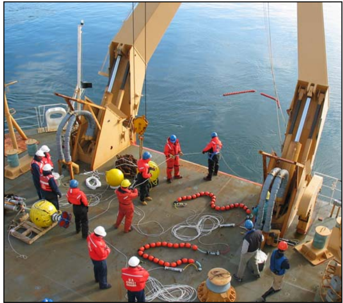
Figure 13. Float strings forming the upper sections of a temperature-salinity mooring are paid out from the stern of the Healy
