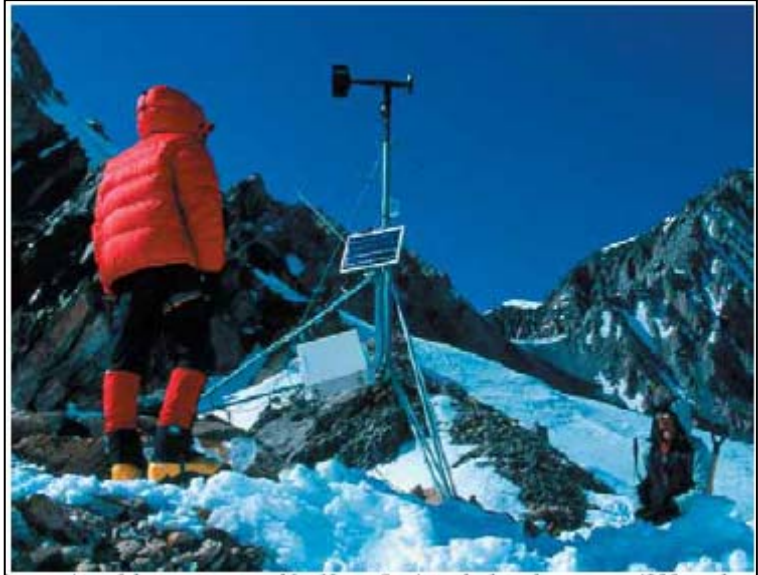
Figure 16. Automatic weather station of the type now operating on Pim Island and at Cape Isabella. This photograph show the same equipment at at 4000 m elevation on Mount Logan.
