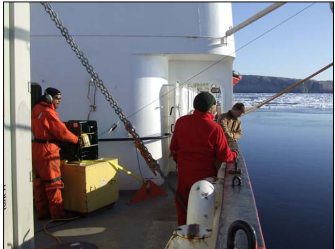
Figure 4. Setup for operating the CTD probe on board CCGS Henry Larsen. CTD deck electronics and the computer for logging data were installed in the 20-foot workshop container seen at the edge of the picture.
