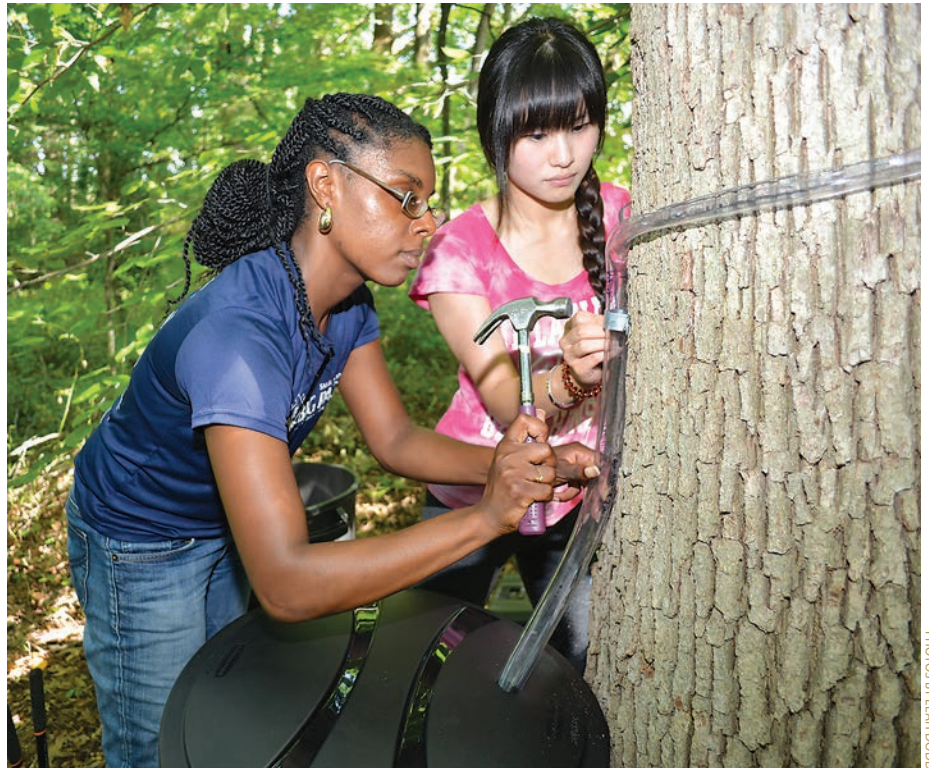
Asia Dowtin and undergraduate student Tianjiao Hao, EG15, install equipment used to measure the rainwater that flows down a tree at a UD research site in Fair Hill, Maryland.
