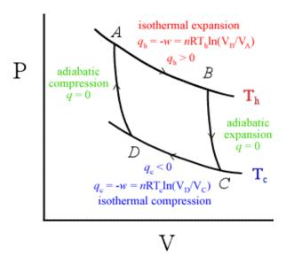
What would the Carnot cycle drawn on a temperature-entropy, T-S, diagram look like? Use temperature for the y-axis and entropy for the x-axis.
