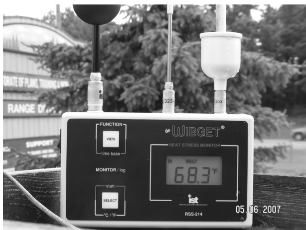
Figure 3. Wet bulb temperature measuring device. Photograph taken by SSG Paul R. Nieman, courtesy of Fort Drum Range Control.
