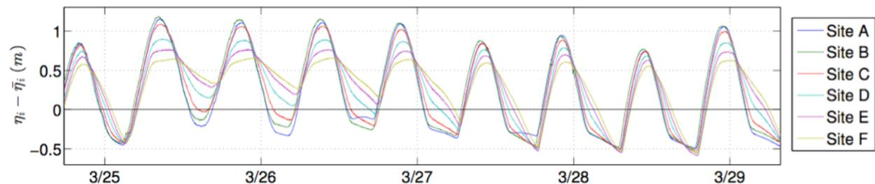
Figure 1. Measured water levels during (3/25 – 3/27) and shortly after (3/27 – 3/29) the surge event, less their respective means, with distance landward increasing from Site A to Site F
