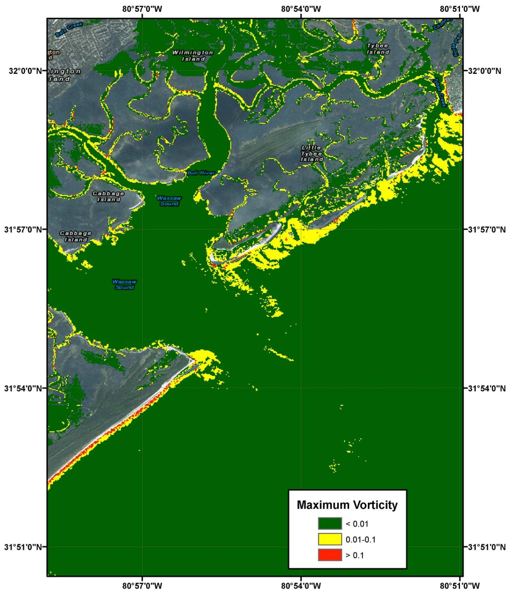
Figure 15: Maximum Vorticity map for Wassaw Sound during CVV80 tsunami
