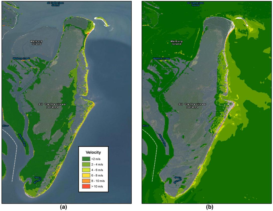
Figure 14: (a) Maximum Velocity map for inundated area around Saint Catherines Island during CVV80 tsunami (b) Maximum Velocity map for Saint Catherines Island during CVV80 tsunami for offshore areas
