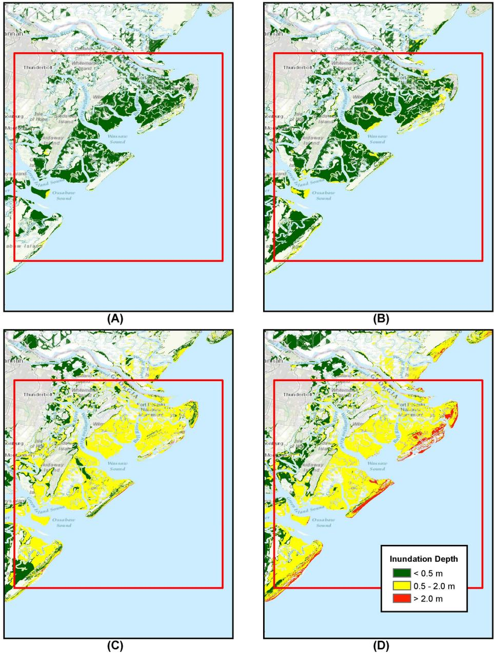
Figure 9: Inundation depth for SA\_1arc\_3 domain, A) SMF, B) Coseismic Envelope, C) CVV 80 km<sup>3</sup> slide, and D) CVV 450 km<sup>3</sup> slide. Red box depicts SA\_1arc\_3 domain boundaries.
