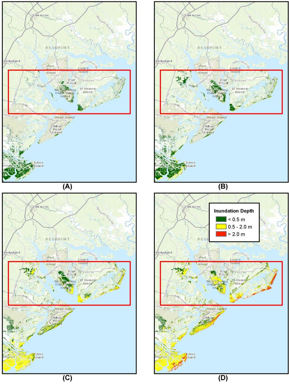
Figure 12: Inundation depth for SA\_1arc\_6 domain, A) SMF, B) Coseismic Envelope, C) CVV 80 km<sup>3</sup> slide, and D) CVV 450 km<sup>3</sup> slide. Red box depicts SA\_1arc\_6 domain boundaries.
