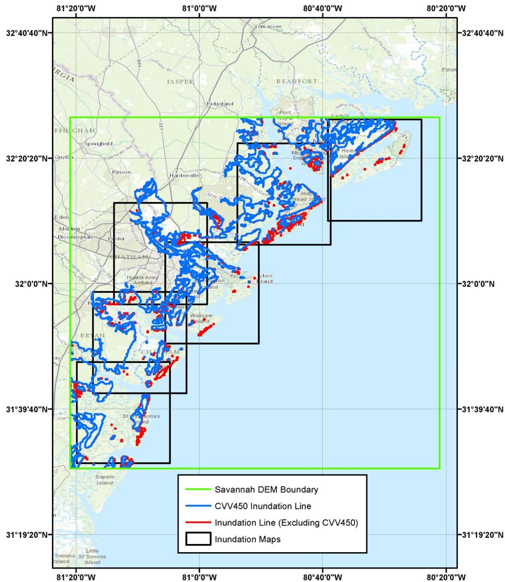
Figure 16: Tsunami inundation line for Savannah NGDC DEM area based on tsunami sources simulated in this project. The red line shows the inundation line for the envelope of all sources excluding CVV450. The blue line demonstrates the CVV450 inundation line. The black boxes show the location of the inundation maps discussed in Section 5.
