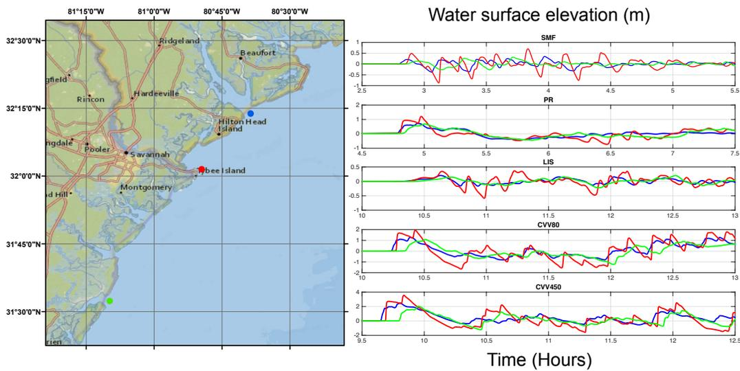
Figure 5: Recorded surface elevation for gauges located in different locations in Savannah DEM, Port Royal Sound (Blue), Savannah River (Red), and Sapelo Sound (Green)
