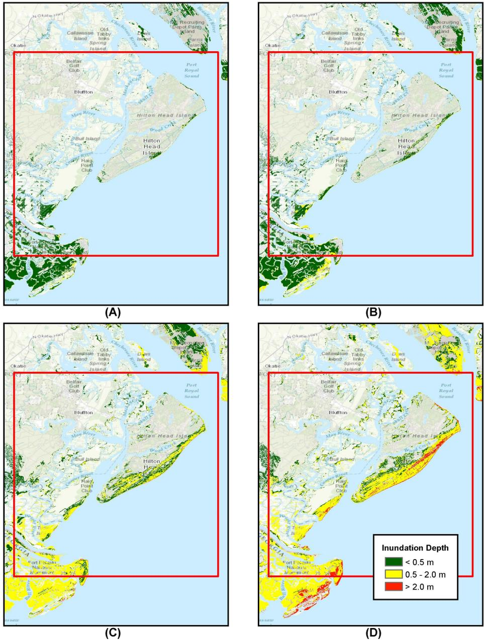
Figure 10: Inundation depth for SA\_1arc\_4 domain, A) SMF, B) Coseismic Envelope, C) CVV 80 km<sup>3</sup> slide, and D) CVV 450 km<sup>3</sup> slide. Red box depicts SA\_1arc\_4 domain boundaries.
