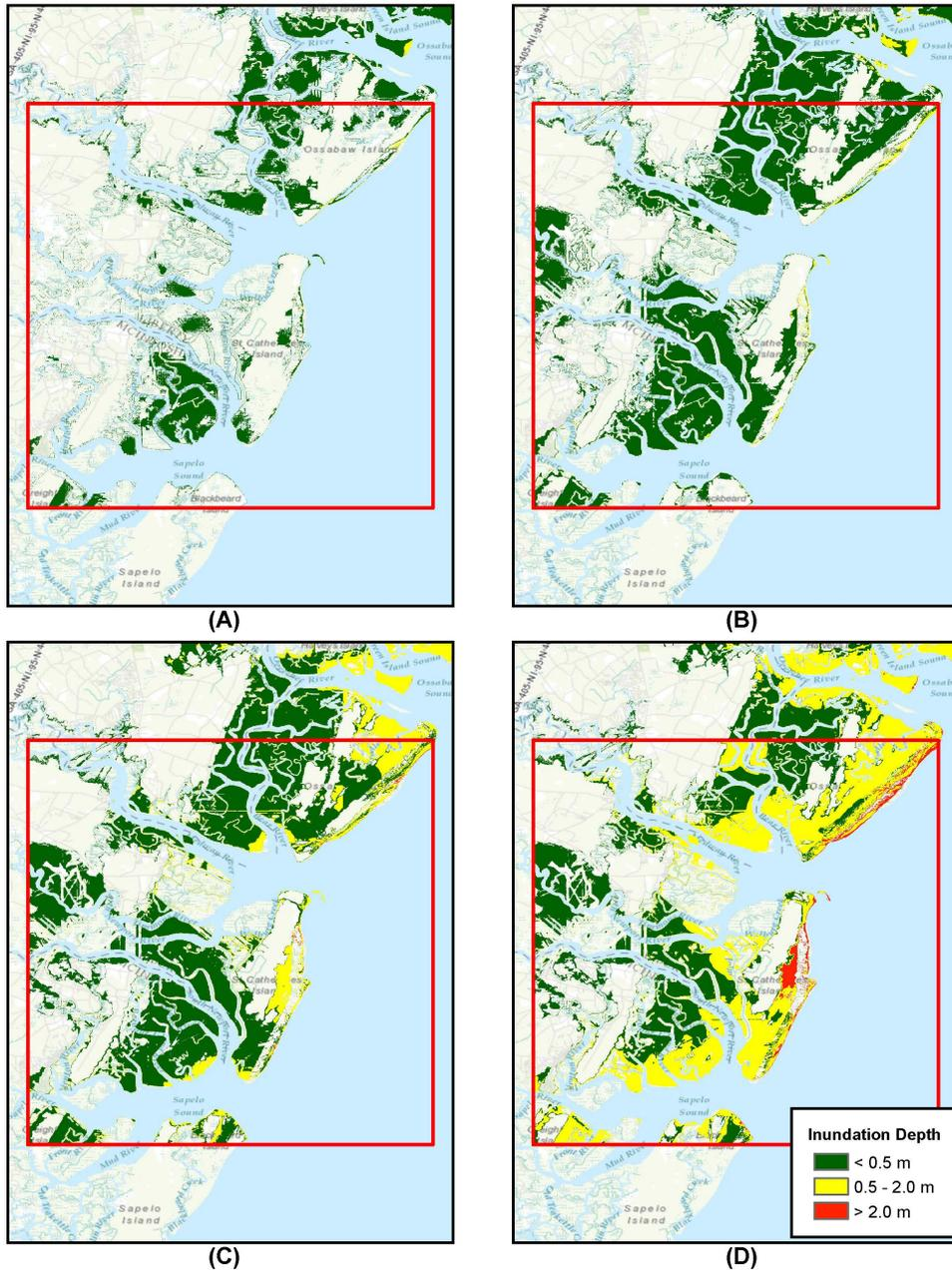
Figure 7: Inundation depth for SA\_1arc\_1 domain, A) SMF , B) Coseismic Envelope, C) CVV 80 km<sup>3</sup> slide, and D) CVV 450 km<sup>3</sup> slide. Red box depicts SA\_1arc\_1 domain boundaries.
