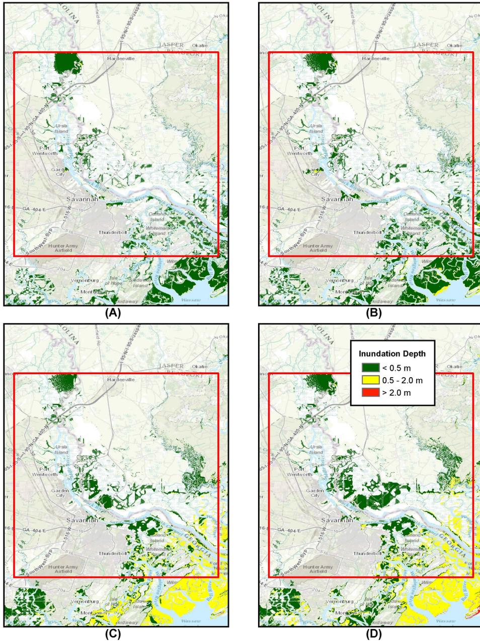
Figure 11: Inundation depth for SA\_1arc\_5 domain, A) SMF, B) Coseismic Envelope, C) CVV 80 km<sup>3</sup> slide, and D) CVV 450 km<sup>3</sup> slide. Red box depicts SA\_1arc\_5 domain boundaries.
