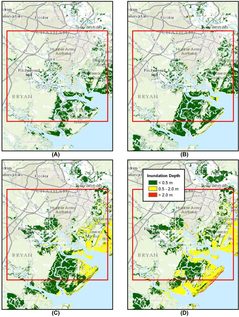
Figure 8: Inundation depth for SA\_1arc\_2 domain, A) SMF , B) Coseismic Envelope, C) CVV 80 km<sup>3</sup> slide, and D) CVV 450 km<sup>3</sup> slide. Red box depicts SA\_1arc\_2 domain boundaries.
