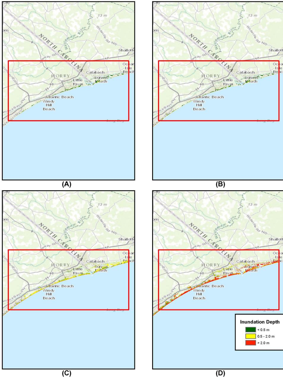
Figure 9: Inundation depth for MB\_1arc\_3 domain, A) SMF, B) Coseismic Envelope, C) CVV 80 km<sup>3</sup> slide, and D) CVV 450 km<sup>3</sup> slide. Red box depicts MB\_1arc\_3 domain boundaries.
