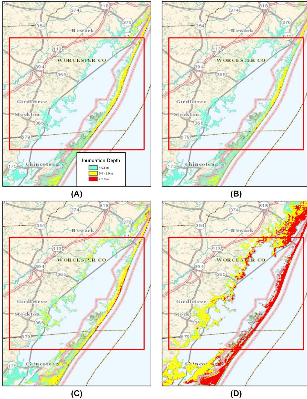
Figure 10: Inundation depth for OC\_1arc\_3 domain, A) SMF Envelope, B) Coseismic Envelope, C) CVV 80 km<sup>3</sup> slide, and D) CVV 450 km<sup>3</sup> slide. Red box depicts OC\_1arc\_3 domain boundaries.
