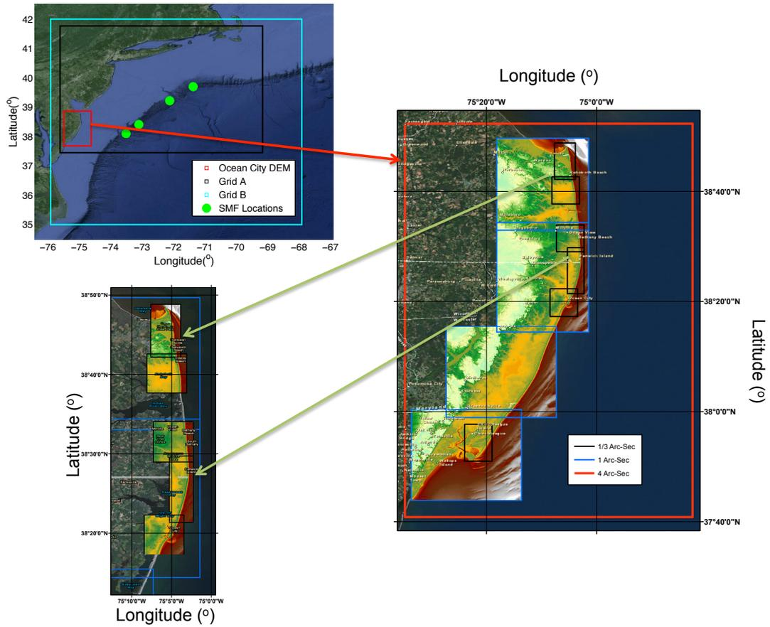
Figure 5: The sequence of grid nesting. The figure on the top left depicts the Grid A and B as well as the location of the Ocean City DEM. The figure on the right show the 1 arc-sec grids described in Table 1. Also, in the bottom left figure the 1/3 arc-sec domains are shown (Also described in Table 1).
