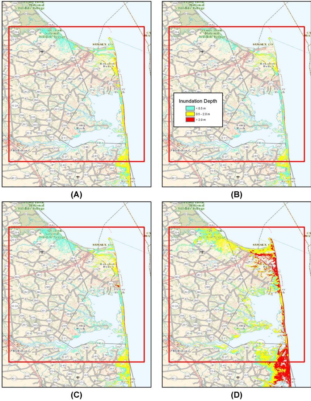
Figure 8: Inundation depth for OC\_1arc\_1 domain, A) SMF Envelope, B) Coseismic Envelope, C) CVV 80 km<sup>3</sup> slide, and D) CVV 450 km<sup>3</sup> slide. Red box depicts OC\_1arc\_1 domain boundaries.
