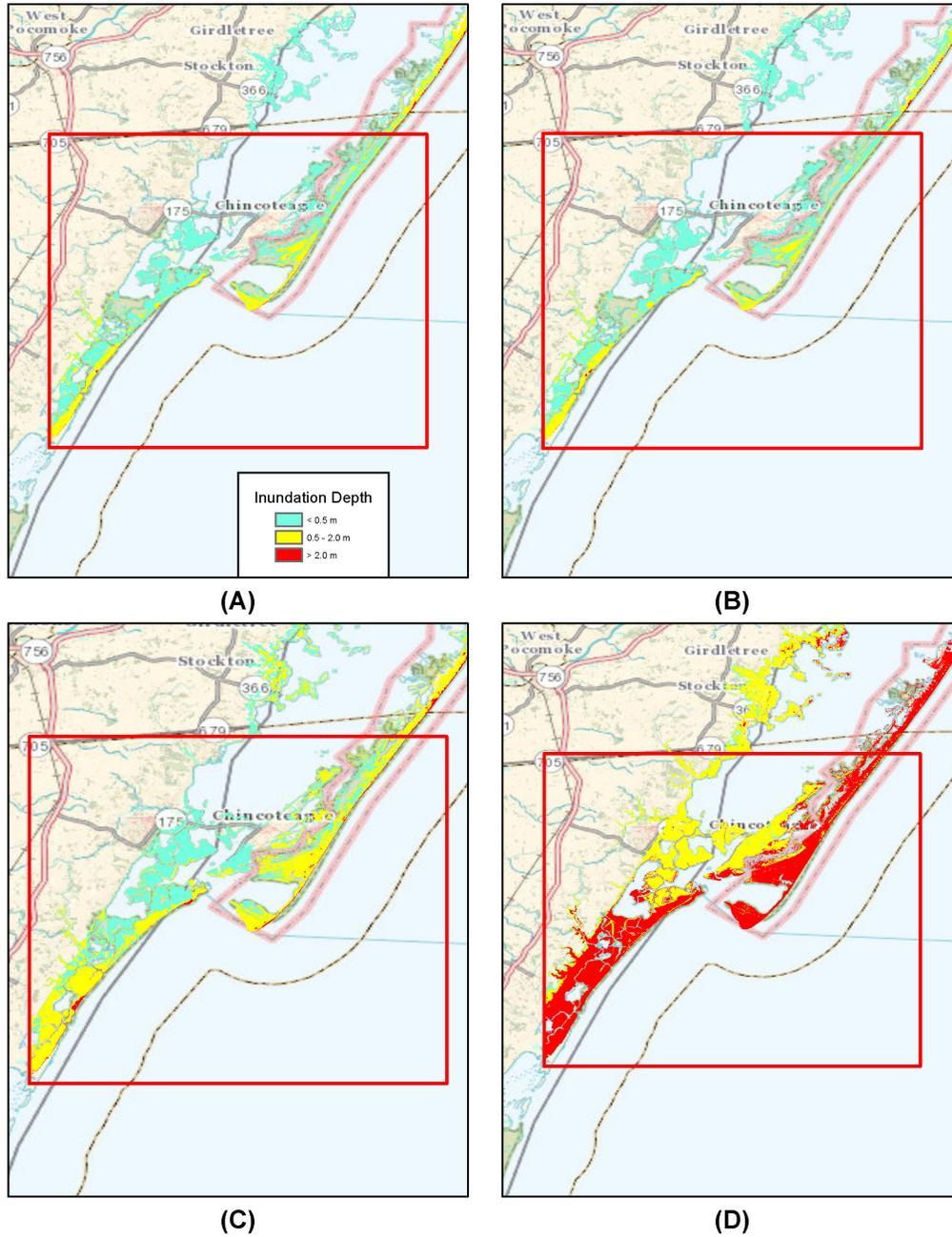
Figure 11: Inundation depth for OC\_1arc\_4 domain, A) SMF Envelope, B) Coseismic Envelope, C) CVV 80 km<sup>3</sup> slide, and D) CVV 450 km<sup>3</sup> slide. Red box depicts OC\_1arc\_4 domain boundaries.
