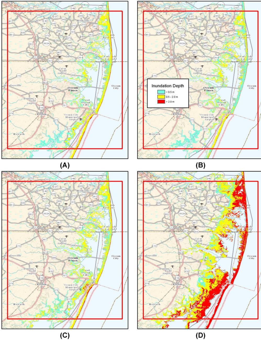
Figure 9: Inundation depth for OC\_1arc\_2 domain, A) SMF Envelope, B) Coseismic Envelope, C) CVV 80 km<sup>3</sup> slide, and D) CVV 450 km<sup>3</sup> slide. Red box depicts OC\_1arc\_2 domain boundaries.
