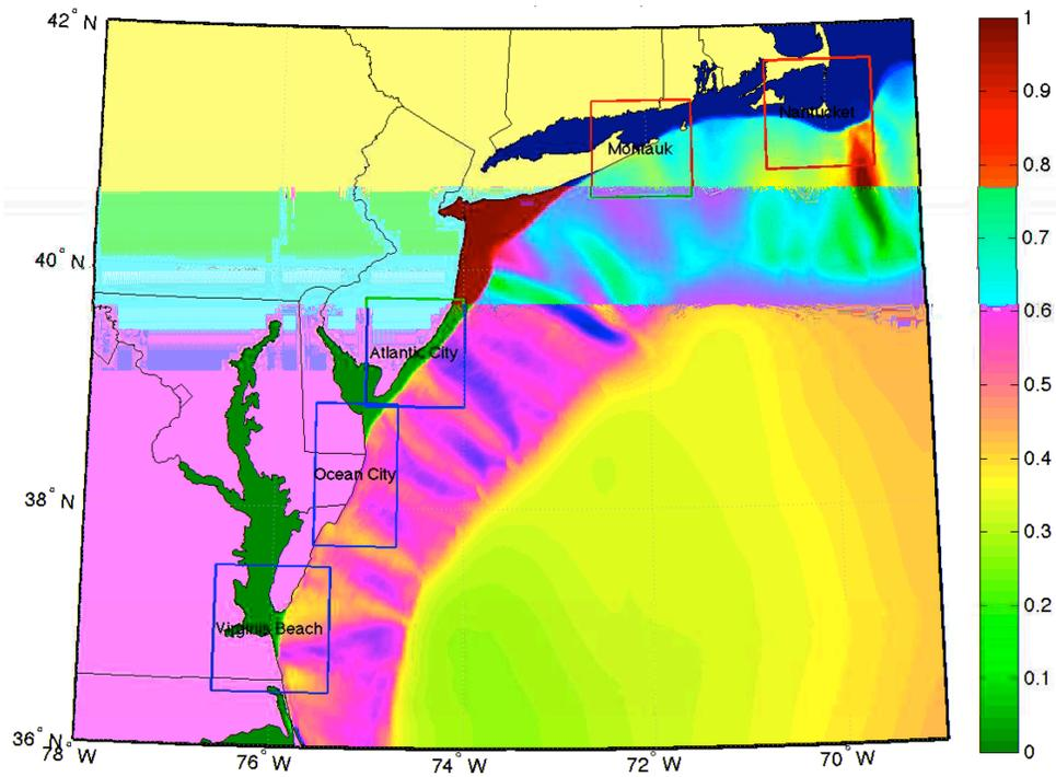
Fig. 10 : Maximum tsunami elevation in a 1' regional grid, for the M 9.0 Puerto Rico Trench source.
