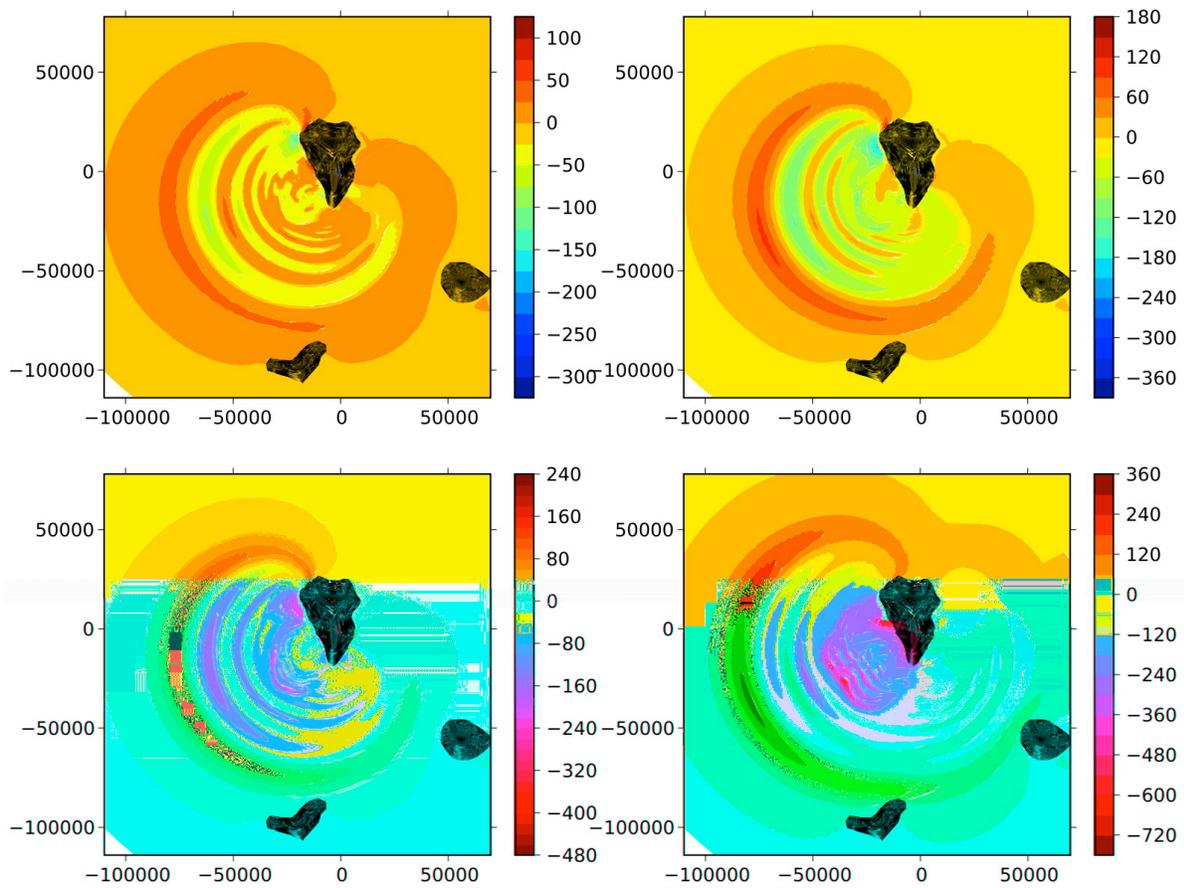
Fig. 5 : THETIS computations in geometry shown in Fig. 4. Computed free surface elevation at  $t = 450 \text{ s}$ , for initial slide volume of: a)  $20 \text{ km}^3$ , b)  $40 \text{ km}^3$ , c)  $80 \text{ km}^3$ , d)  $450 \text{ km}^3$ . [Note the different color scales.]
