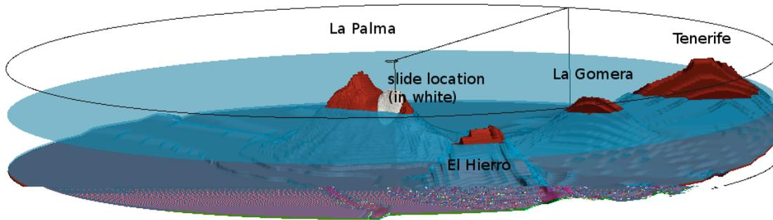
Fig. 4 : Sketch of cylindrical computational domain in THETIS model, for CVV flank collapse simulations, assuming a  $80 \text{ km}^3$  subaerial slide case, with view of bottom bathymetry, neighboring islands, and slide location (marked in white) (Abadie et al., 2011, 2012).
