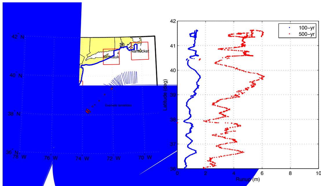
Fig. 8: Right panel: Northern part of runups shown in Fig. 7. Left panel: SMF transects (blue lines) used in MC analysis and location and size of underwater landslides causing 500 year runup (red ellipses). The solid blue line indicates the simplified coastline used in MC simulations and the red boxes mark the size and locations of DEMs currently available from NOAA-NGDC.
