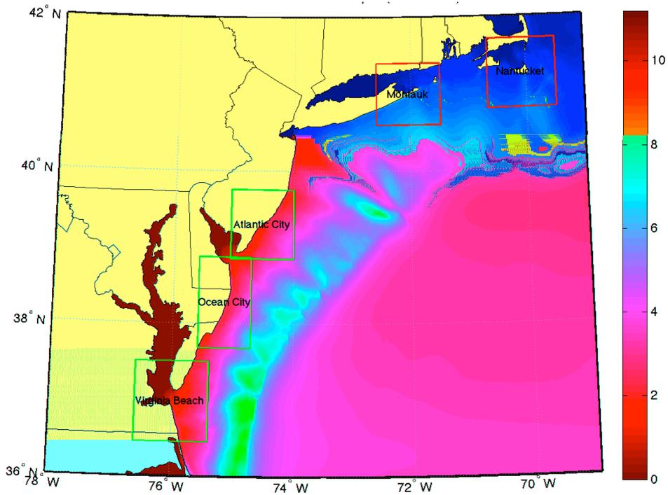
Fig. 11: Maximum tsunami elevation in a 1' regional grid, for the CVV (80 km<sup>3</sup>) source of Fig. 5c
