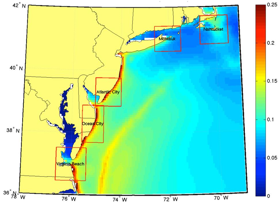
Fig. 9 : Maximum tsunami elevation in a 4' ocean grid, computed for the ACZ sources of Fig. 2.
