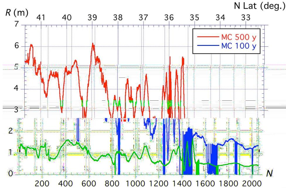
Fig. 7: Runup predicted by MC simulations of SMF tsunamis, for the USEC, for 100-yr. and 500-yr. runup events (Baxter et al., 2011; Krauss, 2011). The bottom x-axis is the index of studied coastal points, numbered N-S and the upper x-axis denotes the latitude (Fig. 6).
