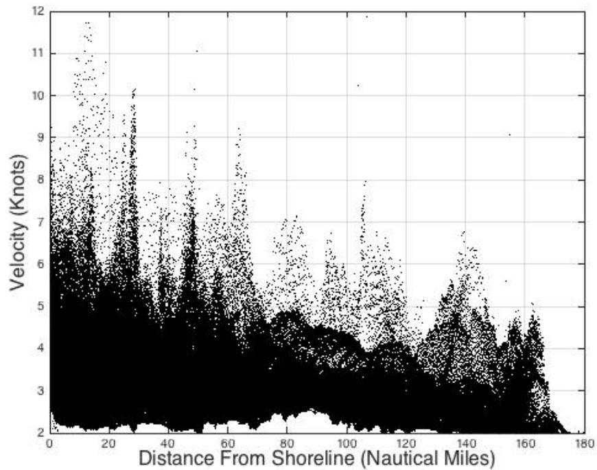
*Figure 3. Maximum occurring velocity at each grid point vs an estimate of offshore distance. Ocean City, MD NGDC DEM (Tehrani-rad et al, 2014).*
