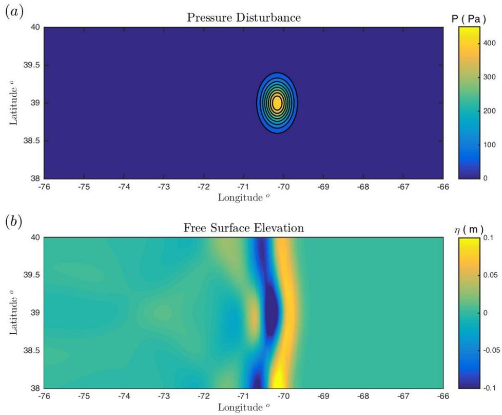
*Figure 5: An idealized meteotsunami example. A Gaussian pressure distribution with major and minor axes = 30 km and central pressure deficit of 450 Pa translates at speed 20m/s over a water body of constant depth 40m. (top) pressure field. (bottom) Surface wave pattern computed by Boussinesq model FUNWAVE. Wave is evolving in a channel bounded by sidewalls at constant latitudes. Distortion in waveform is due to the N-S variation across the grid.*
