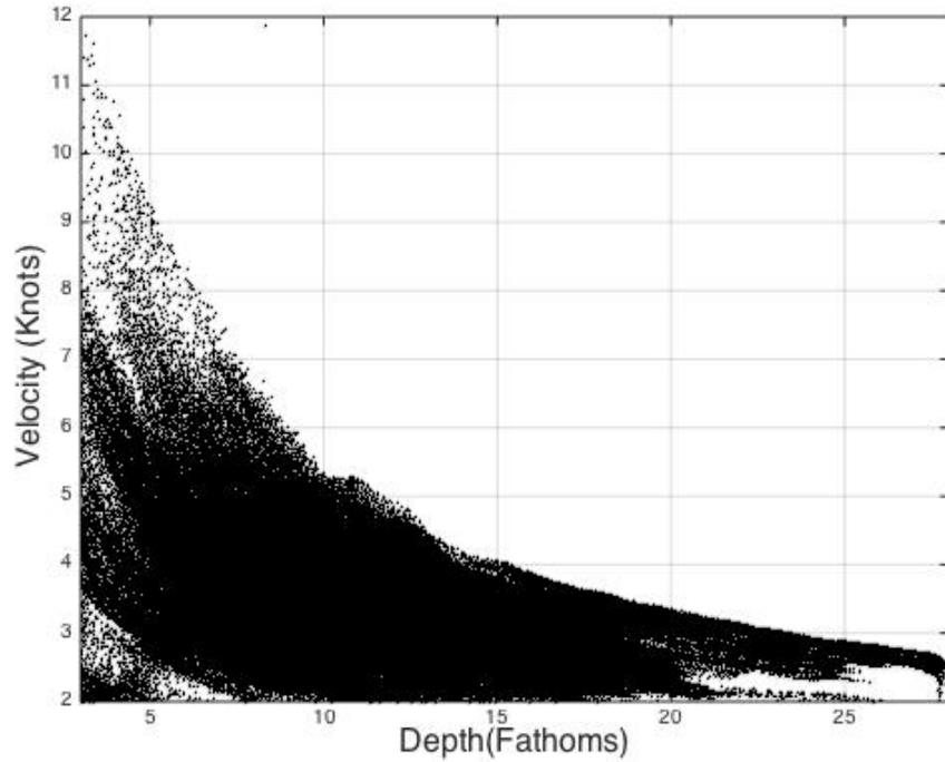
*Figure 2. Maximum occurring velocity at individual grid points as a function of water depth. Ocean City, MD NGDC DEM (Tehrani-rad et al, 2014)*
