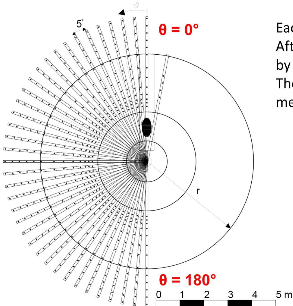
Each experiment is repeated 37 times. After each test the arm has been rotated by  $5^\circ$ . The arm position has been carefully measured by a theodolite.
