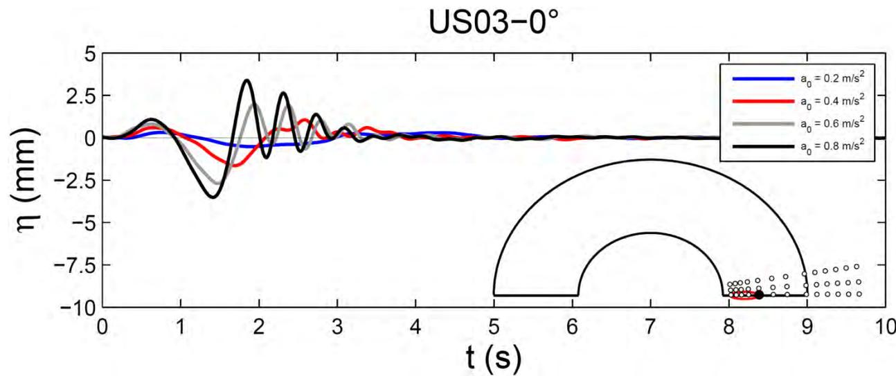
Free surface elevation time series in the near field as a function of the initial acceleration  $a_0$ .
