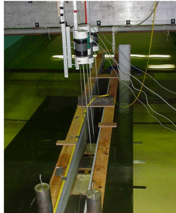
*Wave generation by 2D slide ([Figure 1.1](#)). Experimental set-up, with views of sidewalls, capacitance wave gages, and lead-loaded rolling semi-elliptical slide model*
