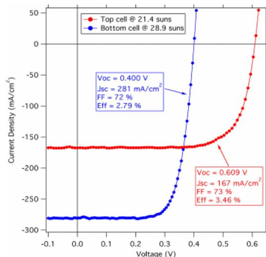
**Figure 12: IV data for the top and bottom subcells of a 3-terminal GaInAsP/GaInAs tandem cell near 20 suns X under an idealized Si filter. The combined efficiencies of the subcells is 6.2%. This solar cell was fabricated by the National Renewable Energy Laboratory (NREL)**
