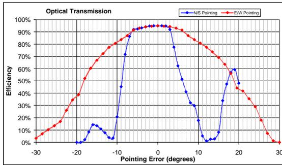
**Figure 5: Optical transmission as a function of angle away from normal to the module.**
