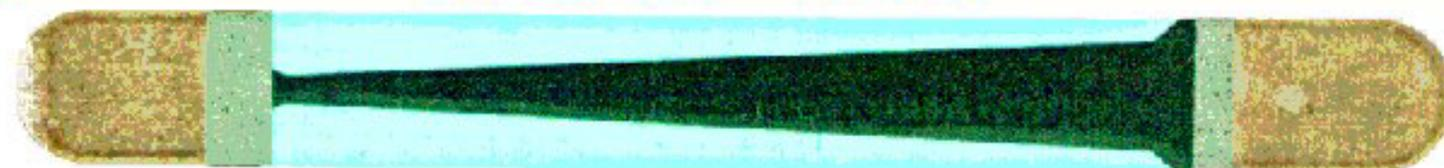
The underside of a Duracell Copper Top AA battery tester is shown in the magnified image above, along with the temperature display that is directly above it. Using simple circuit concepts, explain how this battery tester works.
