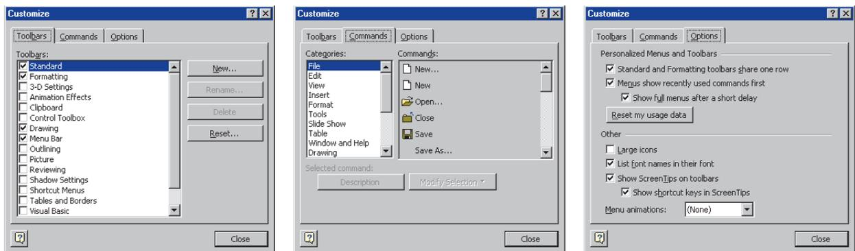
Figure 19-6 The three tabs (Toolbars, Commands, and Options) on the Customize dialog.
