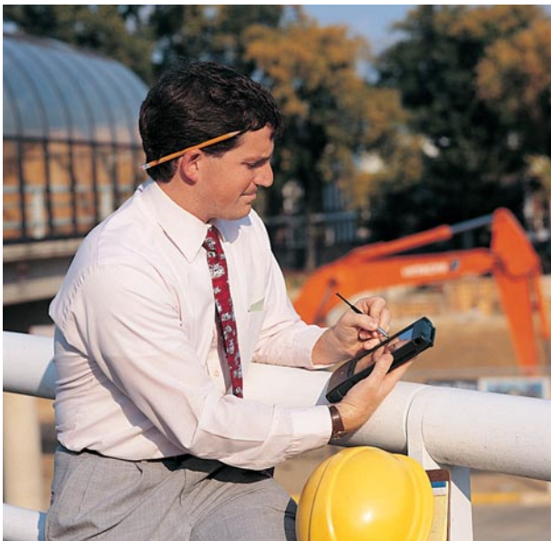
Figure 15-2 Pen computers use a stylus instead of a keyboard to input characters.
