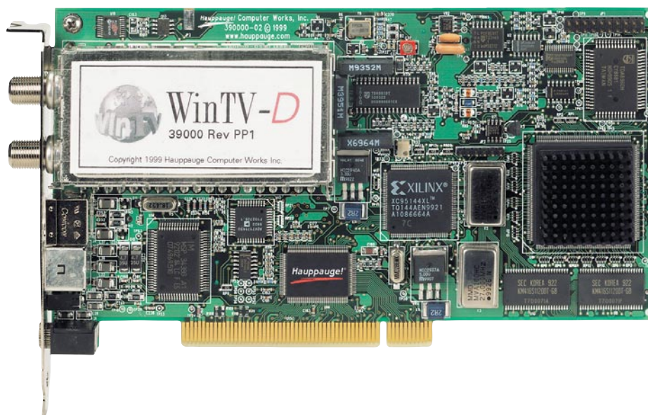
Figure 13-1 The WinTV-pci board has jacks for plugging in a TV cable, video input, and left and right audio channels.
