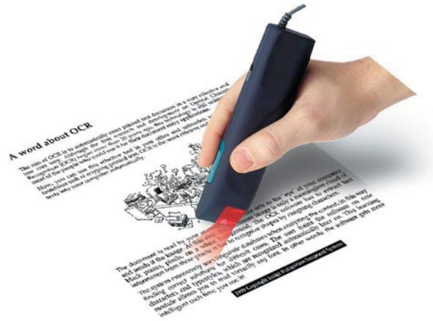
Figure 11-7 The IRISPen scans editable text into the current cursor position.
