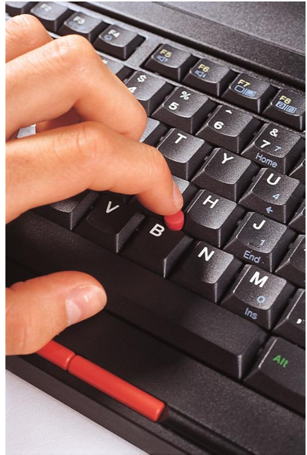
Figure 11-2 A user positions the mouse cursor on the screen with the IBM TrackPoint device.
