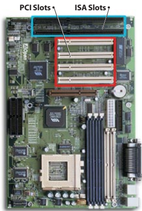
Figure 11-3 On this multi-media PC motherboard, ISA slots are outlined in blue, and PCI slots are bordered by red.
