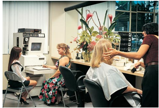
Figure 3-9 The Styles-On-Video system consists of a multimedia computer with video camera, digital video capture card, VCR, pen, and digitizing tablet.
