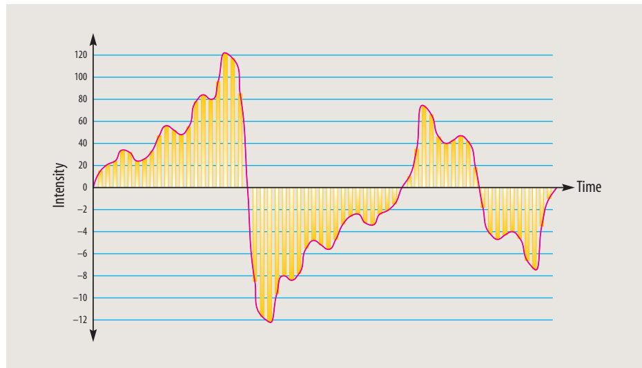
Figure 2-7 Waveform in the process of being sampled; the vertical lines show the points at which samples are taken.
