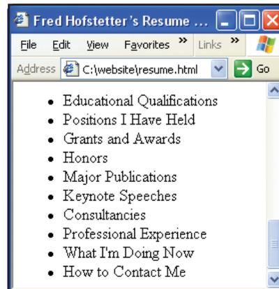
**FIGURE 6-10** This is a browser preview of the HTML in Figure 6-9. Notice that the browser displays the unordered list with bullets. If the list were ordered, on the other hand, the browser would have used numbers instead of bullets. Chapter 8 shows you how to use a style sheet to change the default appearance of bullets, numbers, and other elements onscreen. ■
