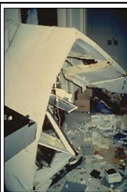
A residential refrigerator explosion due to storage of flammable liquids in the unit
