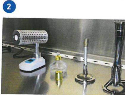
As a result, due to the variable outcome from location to location, and between burner types, it has been concluded that using a heat source within a BSC cannot be recommended!
