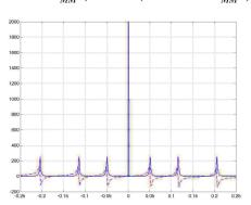
The spectra of the interferograms locate the frequencies of the harmonics comprising the the interferograms. The bands locations are the same, the widths of the bands in the spectra of the decaying interferogram are wider.
