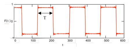
Another way to describe the square wave is as the convolution of a rectangle function and pulse train (comb function). This means that the FT is the product of the sinc function and an inverse (frequency domain) pulse train. The frequency spacing of the pulse train is  $w_0=\pi/T$ .
