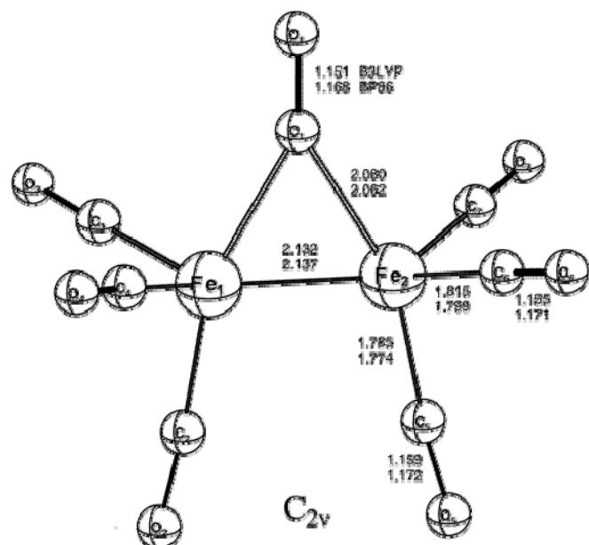
$\text{Fe}_2(\text{CO})_7$  neutral monobridged  $\text{C}_{2v}$  structure optimized using DFT from ref. 1.
