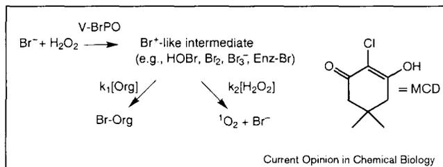
A general scheme for V-BrPO reactivity. When the organic substrate, Org, is monochlorodimedone, MCD,  $k_1[\text{MCD}]$  is competitive with  $k_2[\text{H}_2\text{O}_2]$ . <sup>1</sup>O<sub>2</sub> is formed in the bromide-assisted disproportionation of H<sub>2</sub>O<sub>2</sub> (see reviews [1\*,2,3\*,4\*,5]).
