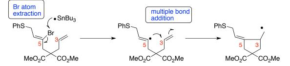
Map out the carbon atoms that you have not yet connected. It becomes apparent that C-6 needs to be connected to C-5. Use a multiple bond addition to accomplish it.
