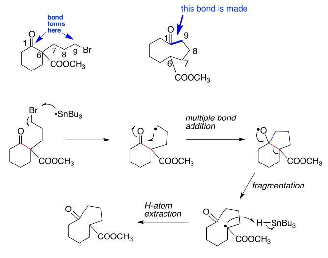
This example illustrates two of these processes: atom abstraction and double bond addition (in this case, an intramolecular version)
