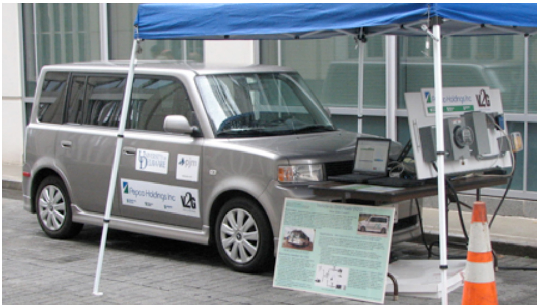
Figure 6: Typical set-up for demonstrations. Here, a Vehicle-to-Grid demonstration at FERC in Washington, D.C. Operating off of the PJM regulation control signal (monitored by the laptop computer), the vehicle showed bidirectional flow of electricity using standard residential electric meter and breaker boxes shown at right.
