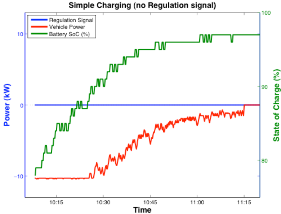
Figure 8: Simple charging, with power flowing from the grid to the vehicle. As the battery reaches full charge, about 10:25, charging current slows and eventually stops at 11:15.
