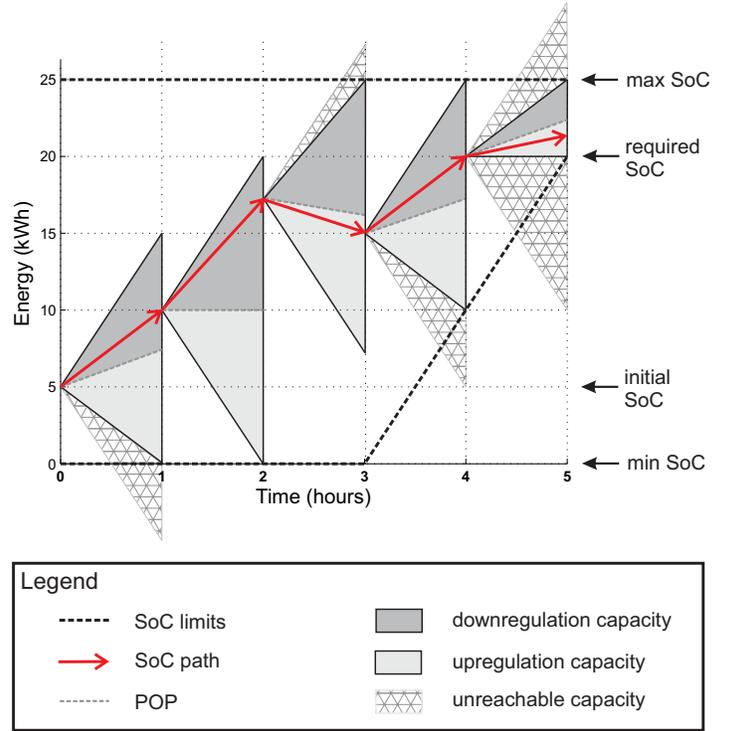
Fig. 4. Example of calculating regulation-up and regulation-down power by a single EV.
