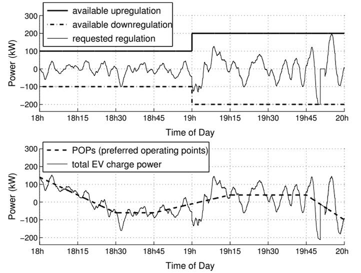
Fig. 2. (a) Regulation bids for two hours, and PJM's resulting online regulation signal. (b) Matching regulation response of the EV fleet, around the POPs.
