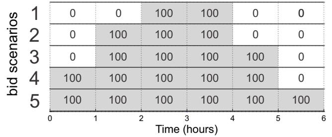
Fig. 6. Different bid scenarios. For each hour in a scenario, the EV aggregator bids for 0 or 100 kW regulation power.
