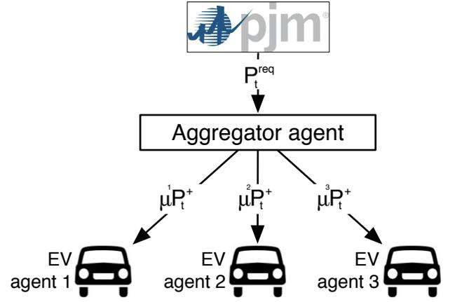
Fig. 3. PJM continuously sends a regulation signal to the aggregator agent, which divides the signal between EVs.
