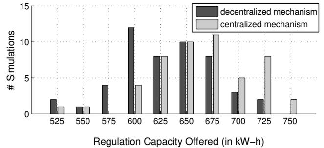
Fig. 9. Regulation maximization without a 100 kW bid restriction (x-axis represents the center of equidistant bins).
